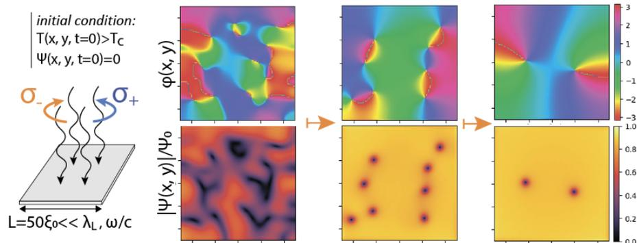
Time evolution of the modulus and phase of the order parameter  $\Psi(x,y,t)$  in a two-dimensional superconductor exposed to an external polarized light with the frequency  $\omega$ . At  $t=0$  the order parameter is equal to zero at each point, so superconductivity is recovered in the presence of an external homogeneous electromagnetic field with  $\sigma_-$  polarization. The sign of polarization determines the sign of vortices remaining in the superconductor.
