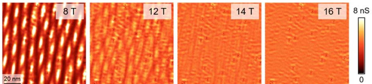
Tunneling conductance images of FeSe at Fermi energy under various magnetic fields applied along *c* axis.
