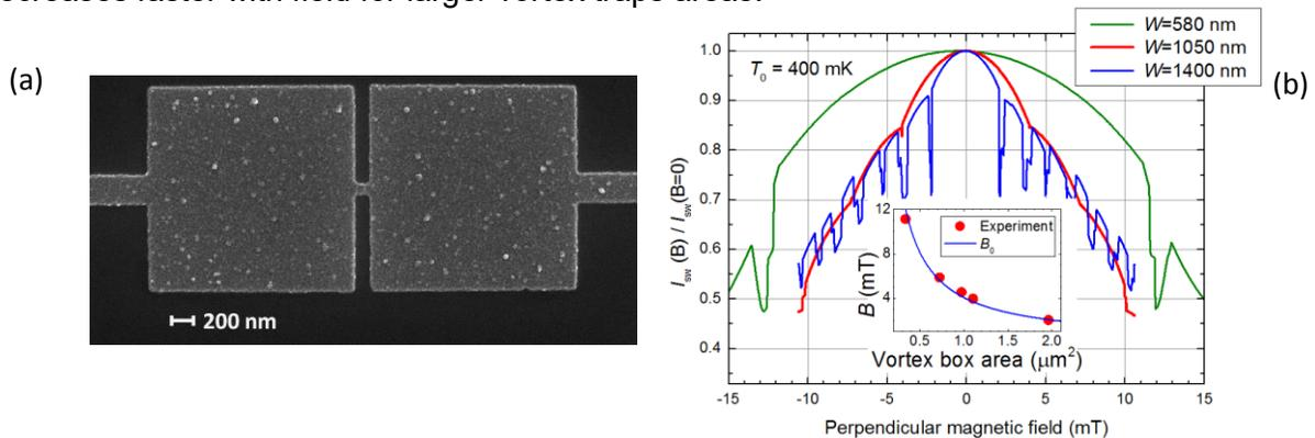
Fig. 1: (a) A typical SEM photo of the vortex traps connected directly to the aluminium Dayem nanobridge. (b) The normalized  $I_{SW}$  vs. perpendicular magnetic field for different vortex trap sizes. Inset: Theoretical and experimental critical fields  $B_0$  vs. vortex trap area.
