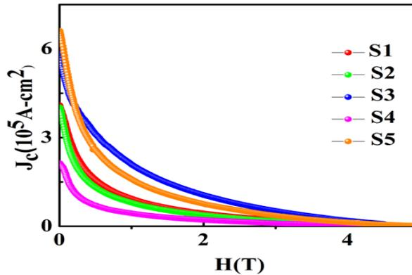
Figure 1: Enhancement in critical current density on increasing the ion (Xe) fluence.
