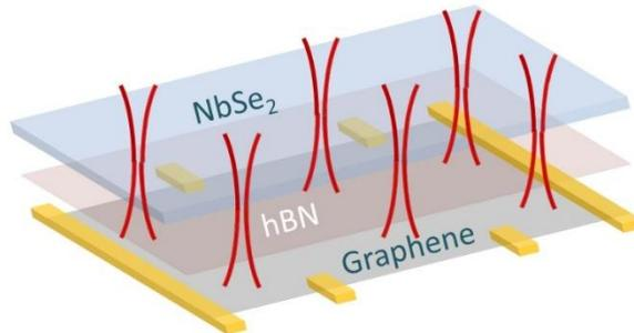
*Device schematic: Abrikosov vortices (red color) are formed in the 40 nm thick NbSe<sub>2</sub> flake and threaded into graphene layer residing at 10 nm (hBN thickness) below the NbSe<sub>2</sub>.*
