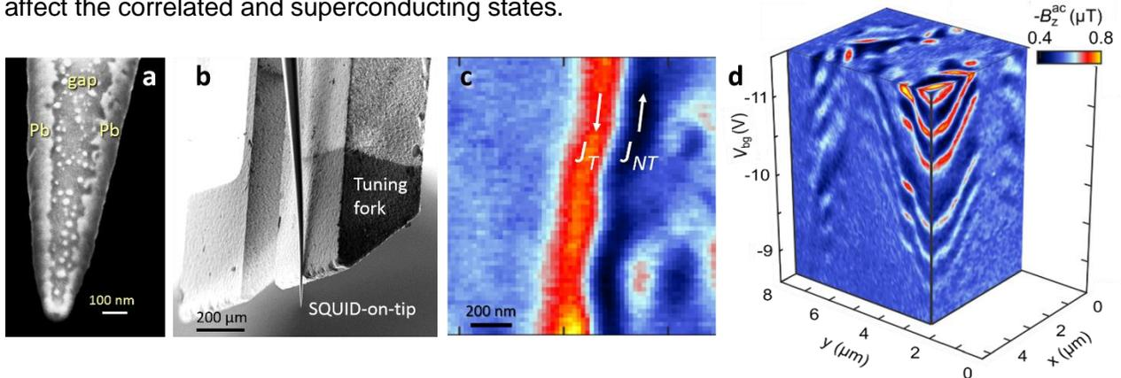
*Fig. 1. (a) SEM image of a Pb SQUID-on-tip. (b) SQUID-on-tip attached to a quartz tuning fork for force sensing. (c) Direct imaging of the counterpropagating topological (red) and nontopological (dark blue) currents flowing in the quantum Hall edge state in graphene at 300 mK and 1 T magnetic field. (d) Tomographic imaging of the equilibrium currents and the Landau levels in magic angle graphene as a function of position and back gate voltage.*
