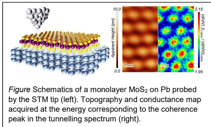
*Figure* Schematics of a monolayer  $\text{MoS}_2$  on Pb probed by the STM tip (left). Topography and conductance map acquired at the energy corresponding to the coherence peak in the tunnelling spectrum (right).
