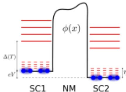
*Insulating potential barrier between two superconductors (boson reservoirs). Here Cooper pairs remain as bound particles in the ground state at energies below the energy gap  $\Delta(T)$  and barrier height  $\phi_0$ .*
