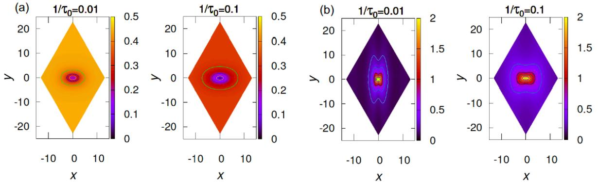
Fig. 1. (a) Pair potential  $|\Delta(\mathbf{r})|$  and (b) zero-energy local density of states  $N(E=0, \mathbf{r})$  around a vortex in a  $p_x$ -wave superconductor for scattering rates  $1/\tau_0 = 0.01$  and  $0.1$  in the Born limit. We show a region within a unit cell of triangular vortex lattice.
