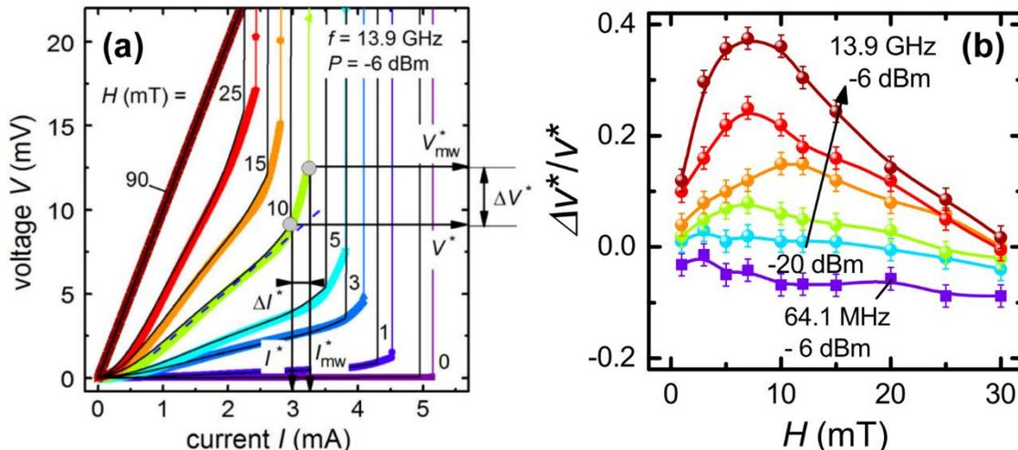
Fig. 1. (a)  $I$ - $V$  curves of a Nb film at a  $T = 0.988T_c$  in the unexcited state (solid lines) and in the presence of a rather high-power-level ac current (symbols). (b) Relative changes of the vortex velocity at the instability point for a series of microwave power levels at 13.9 GHz in comparison with the -6 dBm/64.1 MHz ac excitation.
