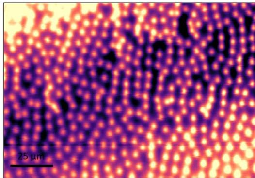
*Scanning SQUID image vortices in 4Hb-TaS<sub>2</sub> at 1.7K*
