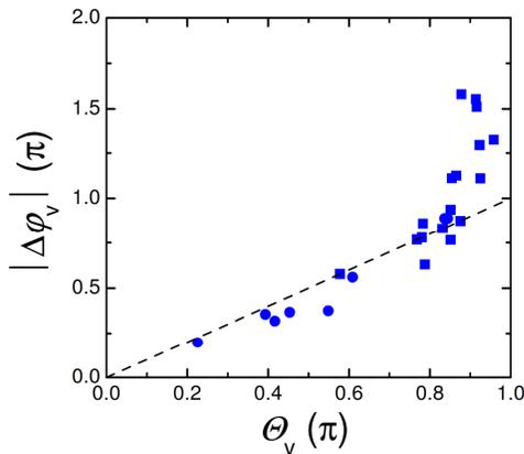
**Figure 1.** Measured Josephson phase shift from a single vortex as a function of the vortex polar angle,  $\Theta_v = 2\arctg(L/2z_v)$ , where  $L$  is the junction length and  $z_v$  is the distance from the vortex to the junction (data from Ref. [3]).
