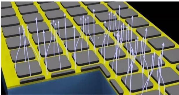
*Schematic of the sample: Nb square islands (grey) form a periodic square lattice (the array). The applied magnetic field penetrates mostly in the gaps between the islands. The Nb islands are placed over a topological insulator film (green) sitting on c-plane sapphire (blue).*
