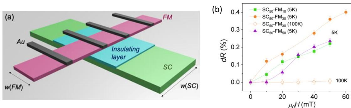
Figure 1. (a) Schematic representation of SC-FM devices. (b) Evolution of the remanent magnetoresistance ratio as a function of the applied magnetic field for different devices at 5K (closed symbols) and 100K (open symbols)
