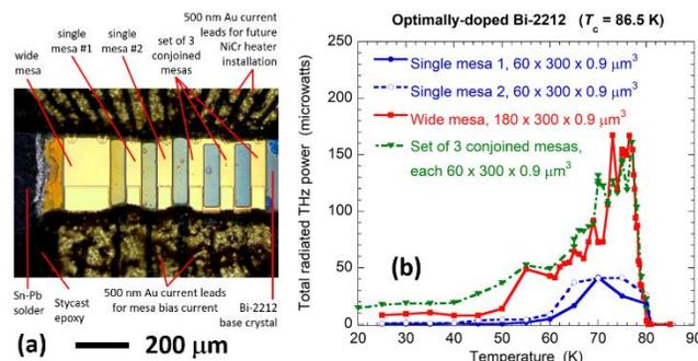
(a) BSCCO THz sources tested in this work. (b) Maximum THz emission as a function of temperature [1].
