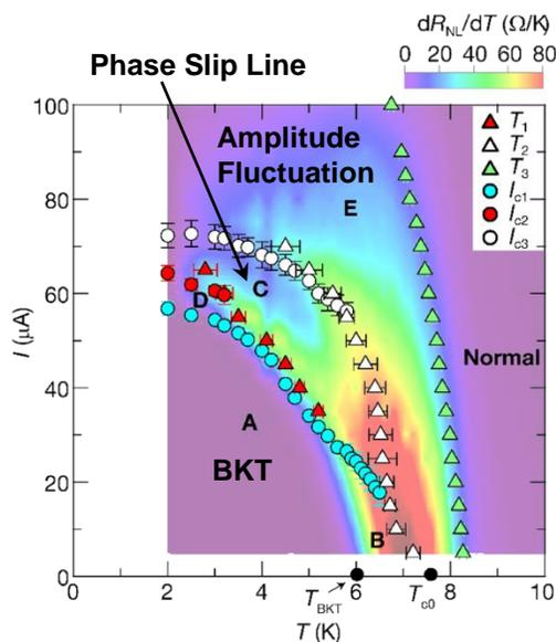
Fig. 1 *I*-*T* phase diagram of ion-gated MoS<sub>2</sub> at zero magnetic field [1].  $I_{c1}$ ,  $I_{c2}$  and  $I_{c3}$ , or  $T_1$  and  $T_2$  are characteristic currents or temperatures at which the step-like increase in *I*-*V* or  $R_{\text{NL}}$  are observed.  $T_3$  is the onset temperature of  $R_{\text{NL}}$ .
