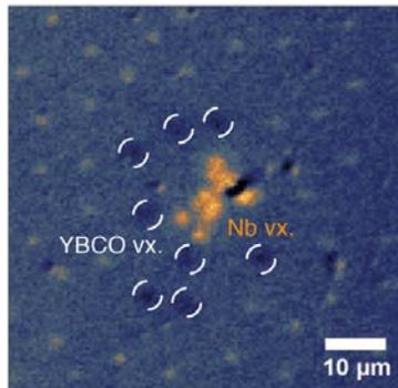
Figure 1. Magneto-optical image of displaced vortices in the niobium film revealing the underlying YBCO vortices
