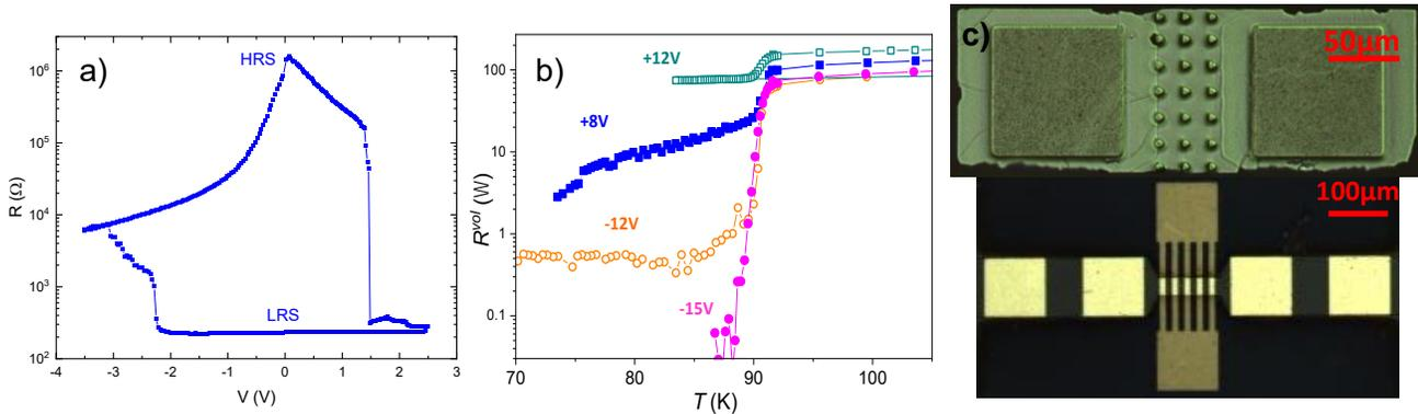
**Figure 1:** (a) Normal state resistance and (b)  $T_c$  modulation through voltage pulses, (c) Different nanostructured contacts patterned in our YBCO track.
