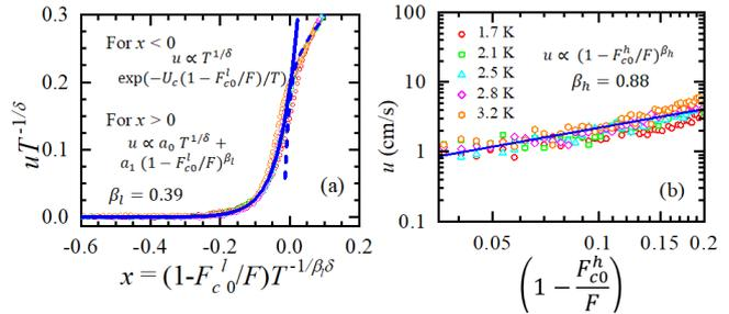
Figure 1: (a)  $uT^{-1/\delta}$  vs  $(1 - F_{c0}^l/F)T^{-1/\beta_l\delta}$  curves estimated from  $I$ - $V$  curves at  $I_c^l$  for various  $T$  and (b)  $u$  vs  $(1 - F_{c0}^h/F)$  curves (in log-log scale) derived from  $I$ - $V$  curves at  $I_c^h$  for various  $T$ .  $I$ - $V$  curves are recorded at 0.7 T. The  $T$ -legends shown in (b) are same for (a). The lines are fitting to the corresponding scaling form.
