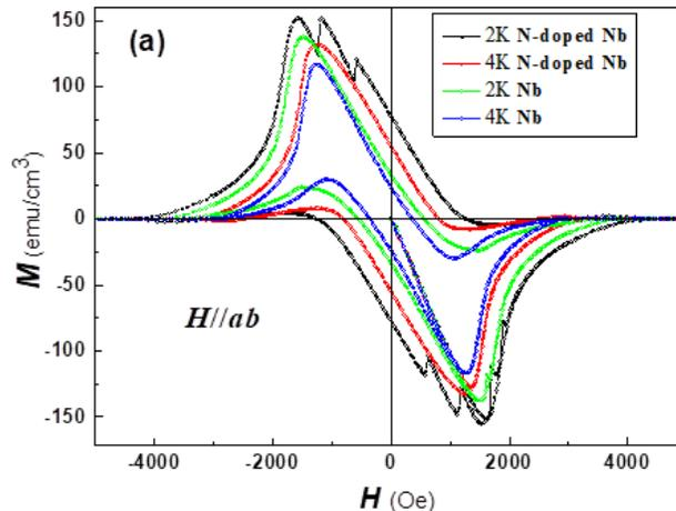
Fig.4(a). Magnetization hysteresis loops (MHLs) of N-doped Nb and pure Nb, with temperatures at 2K, 4K. The applied field  $H_a$  is parallel to the plane.
