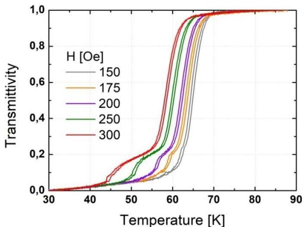
*Transmittivity curves as a function of temperature for different applied fields. Over  $H=150$  Oe the screening happens in two steps separated by a plateau.*
