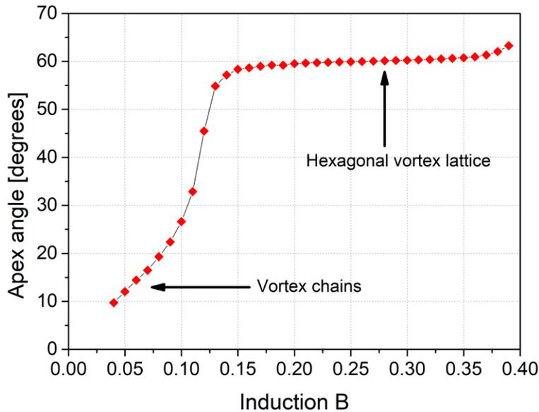
Fig: Equilibrium vortex lattice structure (described by apex angle between primitive vectors of vortex lattice unit cell) as function of magnetic induction  $B$  for  $T = 0.5T_c$  and parameter  $k = 0.8$ . Magnetic field is in units  $\Phi_0/2\pi R^2$  where  $R = v_F/2\pi T_c$ .
