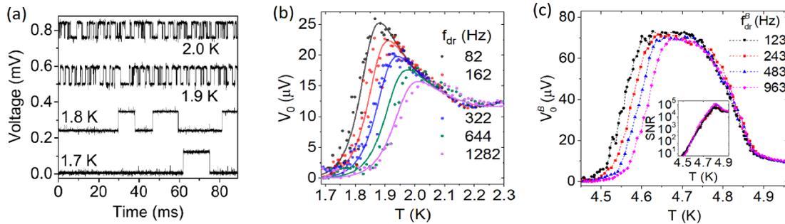
(a) RTN in WL voltage at symmetric bias, (b) Voltage response  $V_0(T)$  for WL at different drive frequencies fitted to two state model of SR, (c)  $V_0^B(T)$  for  $\mu$ -SQUID showing SR with inset showing enhancement of SNR.
