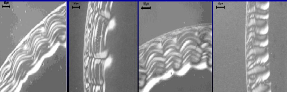
Array of Polymer Droplets by Evaporation of Toluene Layer (70  $\mu$ m) on a Polystyrene Film (43 nm): IITK study
