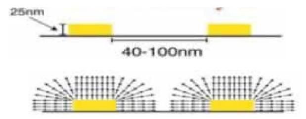
Create gap spacings with multilayer of thiol/carboxylic acid integral multiples of 2 nm layers
