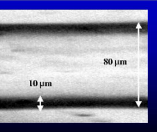
ink-jet printed Copper hexanoate in a volatile solvent
