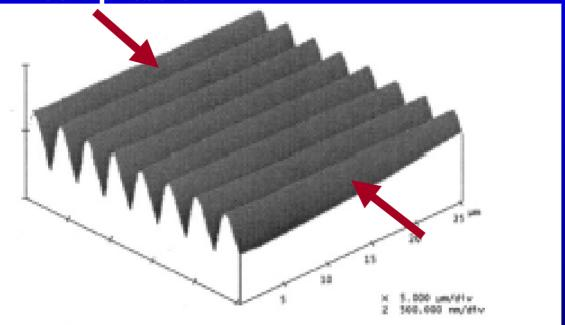
Figure 1. AFM micrograph of a buckled film of polystyrene, having a thickness, h, of 59.7 nm  $\pm$  0.5 nm, supported by and adhered to PDMS.
