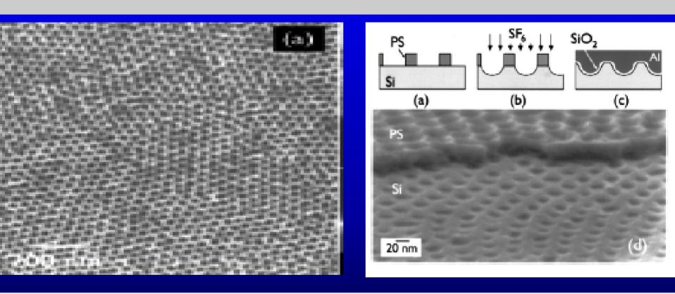
1% solution of PS-PMMA diblock copolymer in toluene spun as a 30 nm thick film; Annealed at 160 °C to make hexagonal lattices of PMMA; 45 nm center-to-center (!) without high resolution lithograpgy techniques; Ultraviolet exposure to cross link PS; removal of PMMA by acetic acid leaving polymer mask; Dry etching of silicon followed by thermal growth of oxide and remaining device processing Black et al., Appl. Phys. Lett. 79, 409, 2001.
