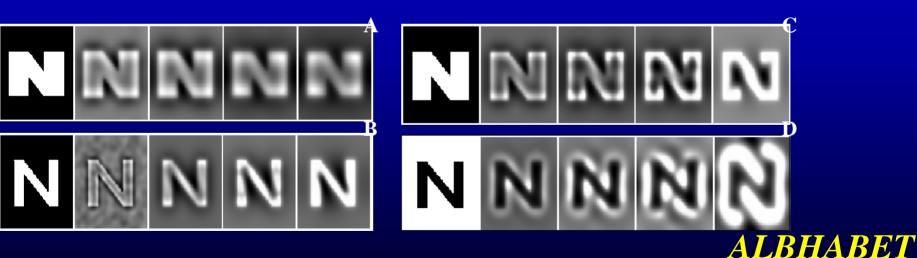
5 nm film. For figs A-D, the pattern "N" is the less wettable part and in fig. D, "N" is the completely wettable part.
