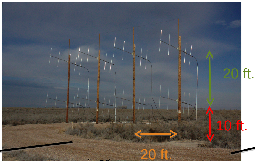
Phased Yagi Array
