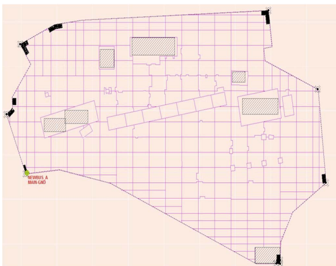
Fig. 4. Top view of hybrid earthing grid
