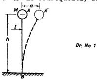
motion, the equation of which we shall determine. No allow ance is made for damping and it is assumed that the displacement a # AA' is within the elastic limit of the struc tural material. The differential equation expressing the motion is :
