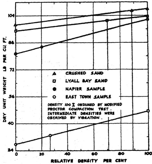
Fig. 1 (c) Results of Relative Density Tests.
