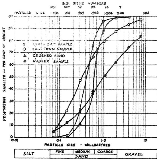
Fig. 1 (a) Soil Tests for Particle Size Distribution.
