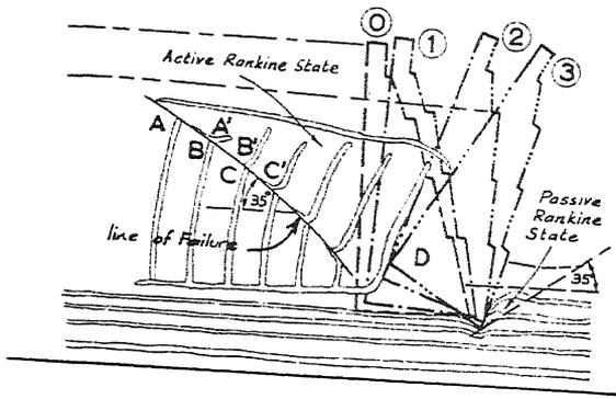
Fig. 16 Diagram showing development of failure of Gravity Wall.
