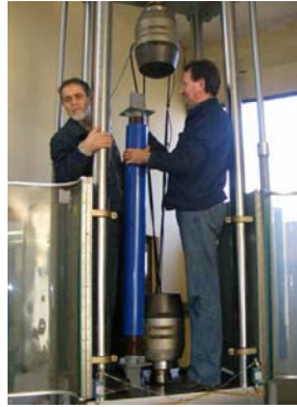
Figure 4. Typical dampers of DC 90 system
