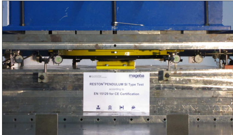
Figure 7. Pendulum Mono isolator during “Type” testing at EUCENTRE
