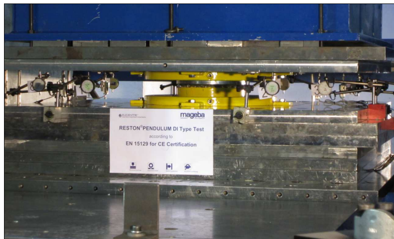
Figure 8. Pendulum Duplo isolator during “Type” testing at EUCENTRE
