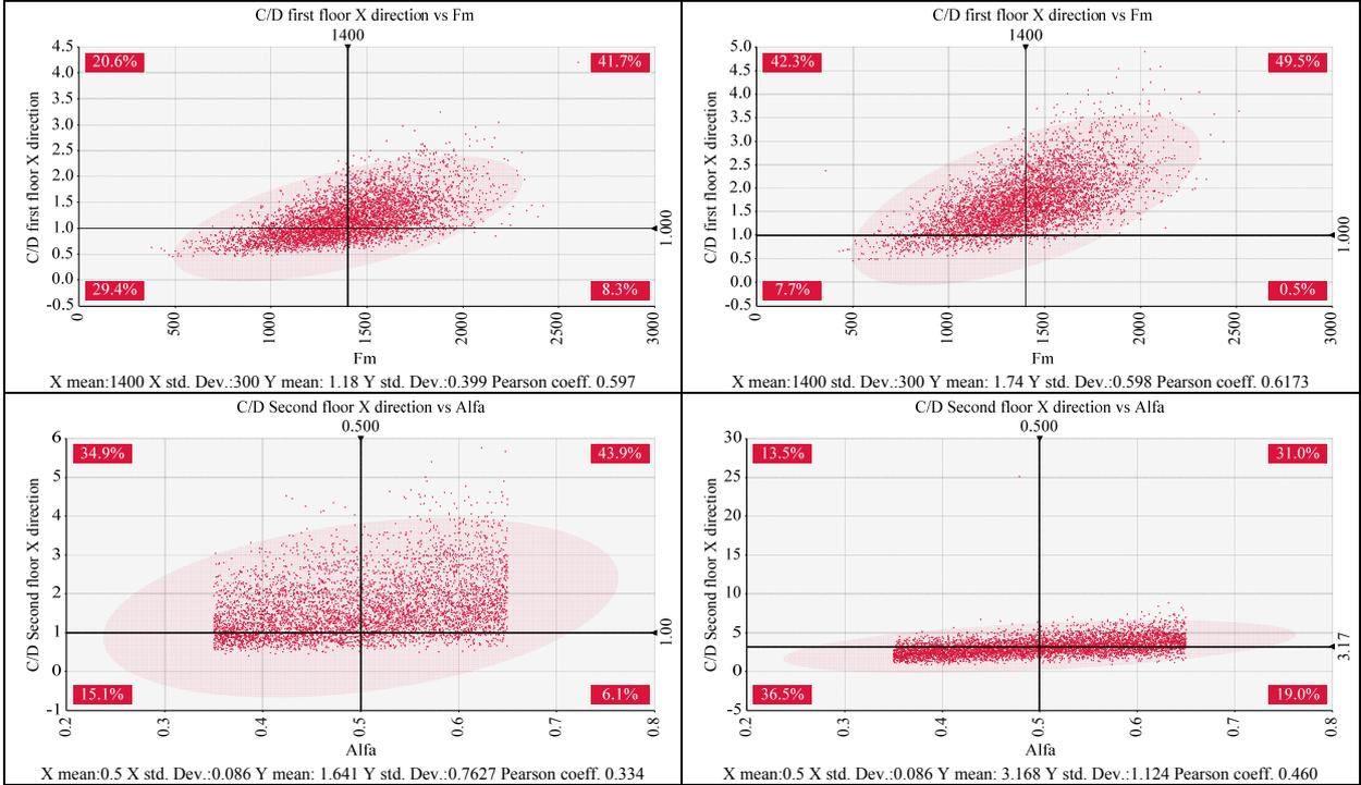
**Figure 6.2.** SU 1: scatter graphs of most influential variables on C/D ratio in X direction for each plane, by starting from first floor on the top line. Section I on the left ( $\eta= 0$ ) and section T on the right ( $\eta= 1$ ).
