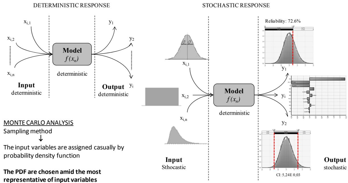
Figure 1.1. – Scheme of the deterministic (left) and of the probabilistic assessment procedure (right).
