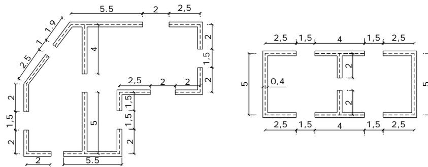
**Figure 6.1.** Example cases: at the left the SU with two floors, at the right the SUs with 3 and 4 floors and the same plan. X direction is horizontal, Y direction is vertical.
