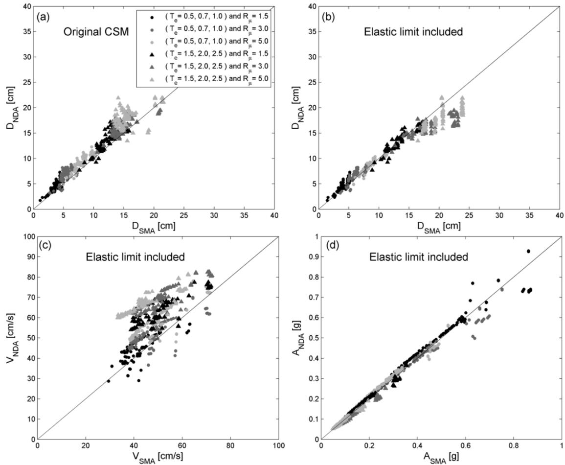
**Figure 4.2.** Approximate methods versus exact response for systems with hysteretic dampers with 2% post-yielding stiffness ratio.
