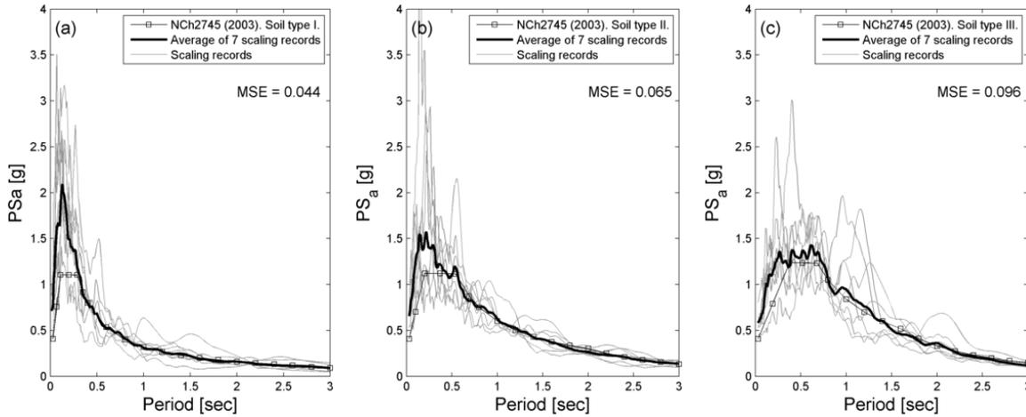
**Figure 2.1.** Average response spectra of the scaled records for soil type: (a) I, (b) II, and (c) III.
