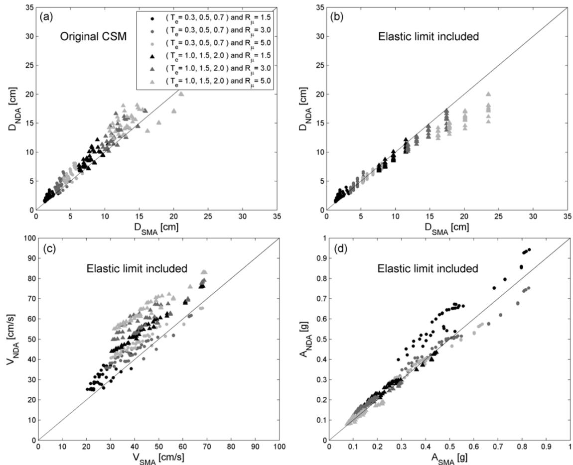
**Figure 4.1.** Approximate method versus exact response for systems with non-linear viscous dampers for  $\alpha=0.6$ .
