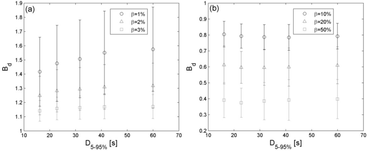
**Figure 3.3.** DMF as function of the significant duration of motion in (a)  $\beta < 5\%$  and (b)  $\beta > 5\%$ .
