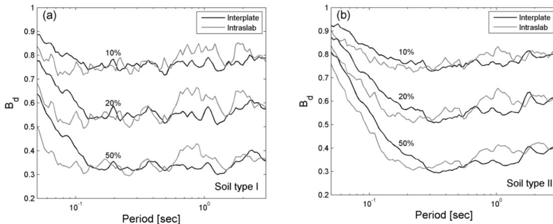
**Figure 3.2.** DMF for inter-plate and intra-plate earthquakes in: (a) soil type I and (b) soil type II.
