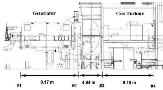
**Figure 5.** Overview of the equipment for Configuration 2, showing bearing locations #1 to #4.
