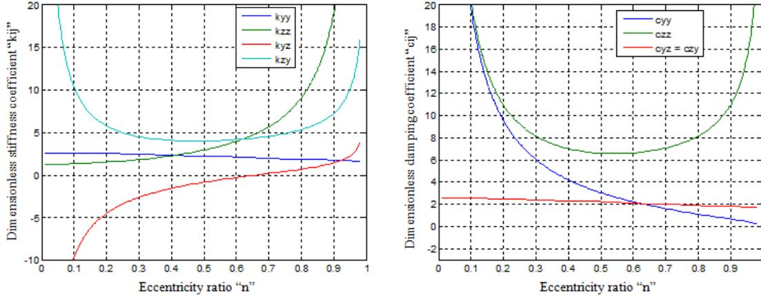
**Figure 1.** Dimensionless coefficient for oil film bearing using the “short bearing” approximation
