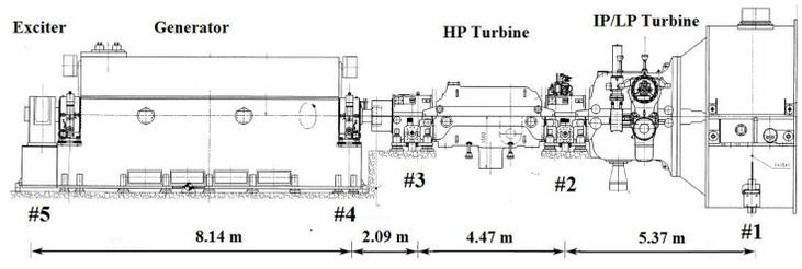
**Figure 7.** Overview of the equipment for Configuration 3, showing bearing locations #1 to #5.
