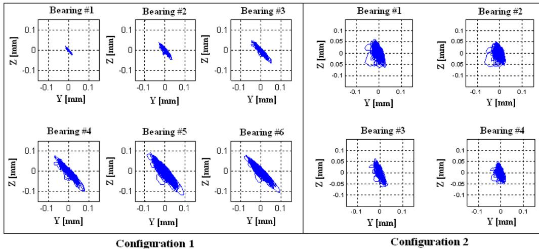
Figure 9. Relative displacement orbits of the rotor in the bearing, Configuration 1 and 2
