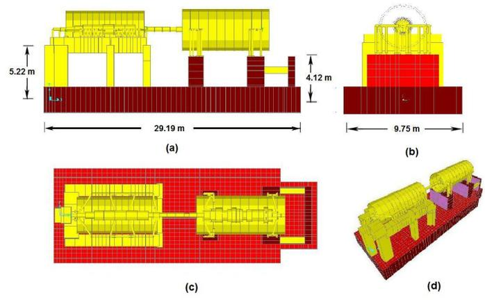
**Figure 6.** Overview of the foundation model for Configuration 2. (a) Longitudinal Elevation, (b) Transverse Elevation, (c) Plan view from above, (d) 3D Perspective. Vertical Figure shows bearing locations #1 to #4.
