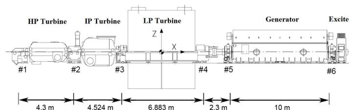
**Figure 3.** Overview of the equipment for Configuration 1, showing bearing locations #1 to #6.
