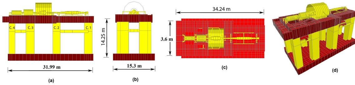
**Figure 4.** Overview of the foundation model for Configuration 1. (a) Longitudinal Elevation, (b) Transverse Elevation, (c) Plan view from above, (d) 3D Perspective
