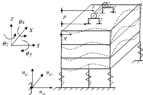
**Figure 2.** Schematic representation of coordinates (degrees of freedom) used to represent the complete system
