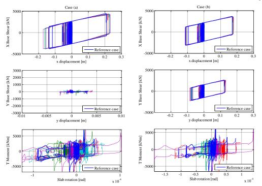
Figure 15. Base forces of the whole system, case a (x-motion, left) and case b (35°-motion, right)
