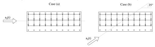
Figure 10. Considered directions of earthquake occurrence
