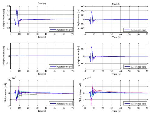
Figure 12. Displacements of the slab versus time, case a (x-motion, left) and case b (35°-motion, right)
