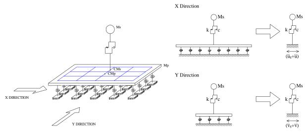
Figure 7. Modelling of the building using an equivalent SDOF per each direction
