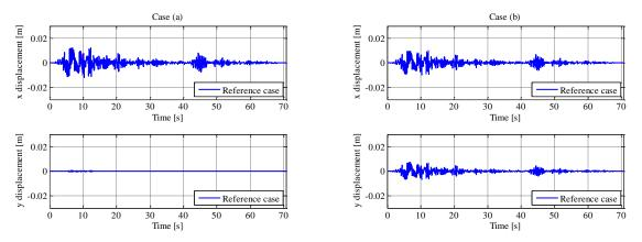
Figure 13. Relative displacements of the building (M<sub>s</sub>) with respect to the base slab versus time, case a (xmotion, left) and case b (35°-motion, right)
