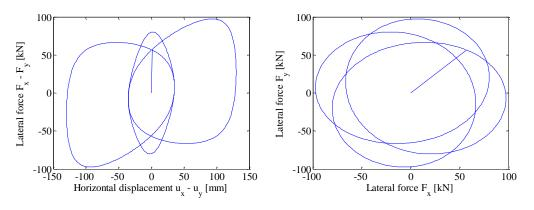
Figure 6. Bi – directional hysteretic behaviour of the device
