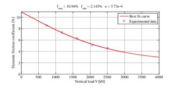
Figure 4. Dynamic friction coefficient versus vertical load: calibration of experimental results
