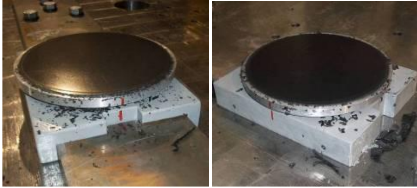
Figure 3.2 Sliders of devices CAR77-1 (L-SlideB, left) and CAR77-3 (L-SlideCF, right) after the test
