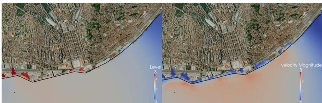
**Figure 5.3.** Low tide simulation. Water elevation (left) and velocity (right) at Baixa waterfront 20 min after hitting Bugio.
