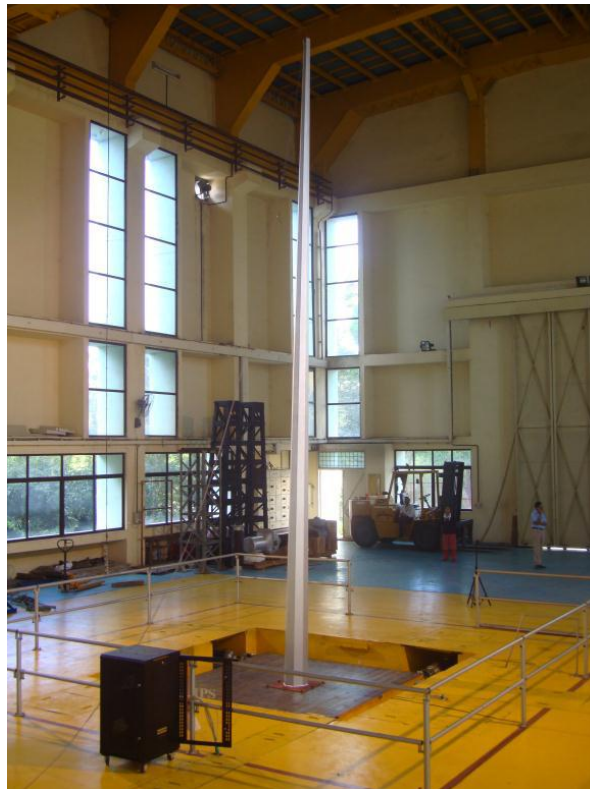
Figure 3.1. Steel pole mounted on shake table
