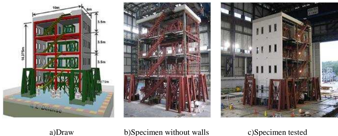
Figure 2. Steel frame tested in the E-Defense
