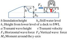
Figure 2.3. Parameters on a tsunami wave load
