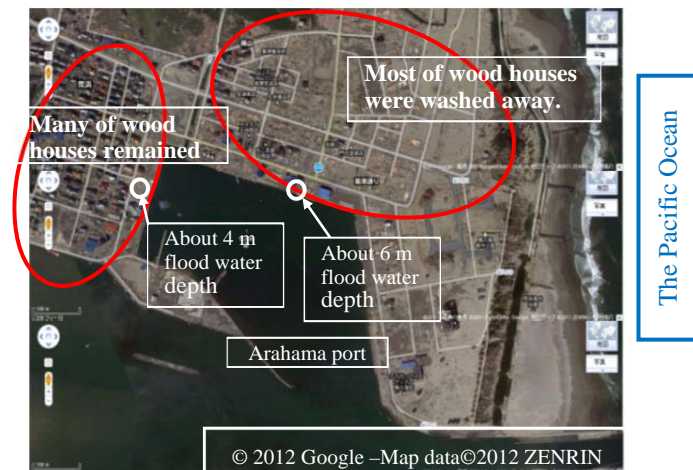
Figure 2.2. Aerial photograph and the flood water depth estimated in Arahama, Watari town.
