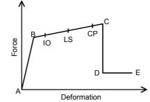
Figure 2.2. Force-Deformation relationship of a typical plastic hinge
