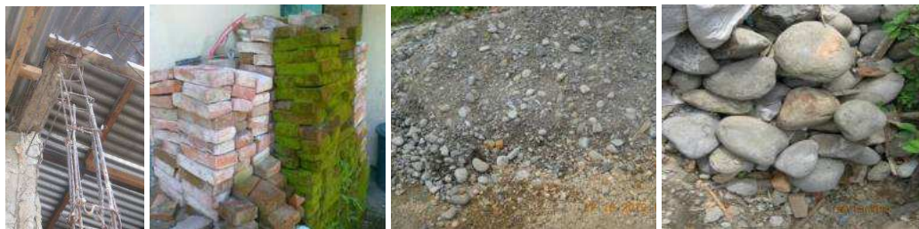
Figure 11: Yielded rebar, lichens in brick, poor aggregate & round-shaped pebble (left to right)
