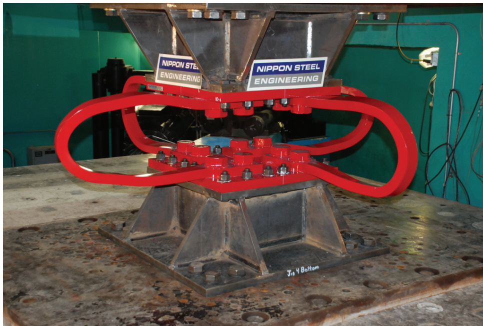
Figure 2. A four-arm U-shaped damper assembly in the UC San Diego, SRMD test machine
