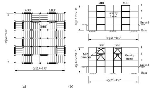
Figure 2.1. Prototype 3-story building structure for real-time hybrid simulations: (a) floor plan; (b) elevation
