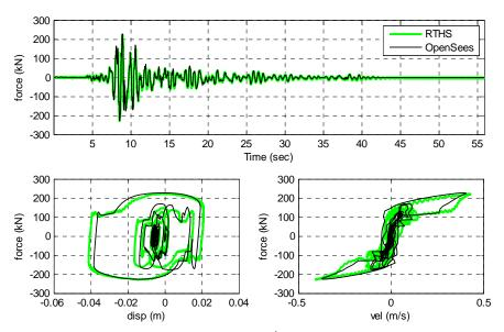
Figure 6.3. Comparison of the 3<sup>rd</sup> story MR damper response (Duzce ground motion; LQR Control)
