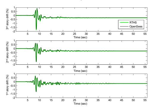
Figure 6.1. Comparison of story drifts between RTHS and OpenSees; Duzce EQ ground motion, LQR control
