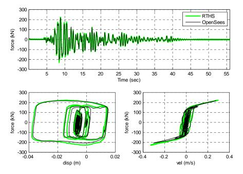
Figure 6.2. Comparison of the 2<sup>nd</sup> story MR damper response (Duzce ground motion; LQR Control)
