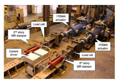
Figure 3.3. Experimental substructure with two MR dampers
