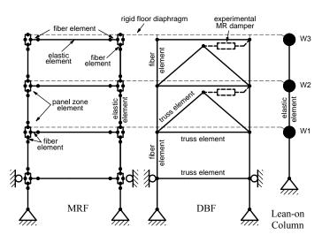
Figure 3.2. Analytical substructure model for real-time hybrid simulations (dampers of experimental substructure indicated for clarity)
