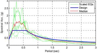
Figure 5.1 Response spectrum of ground motions scaled to DBE
