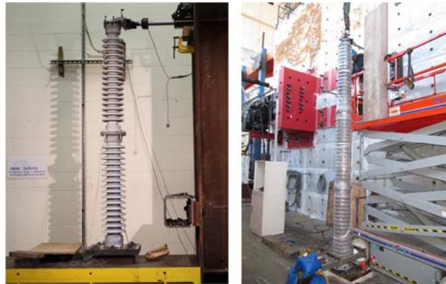
Figure 2.1 Cyclic-loading and fragility test setups used for 230-kV (left) and 550-kV (right) insulator posts.
