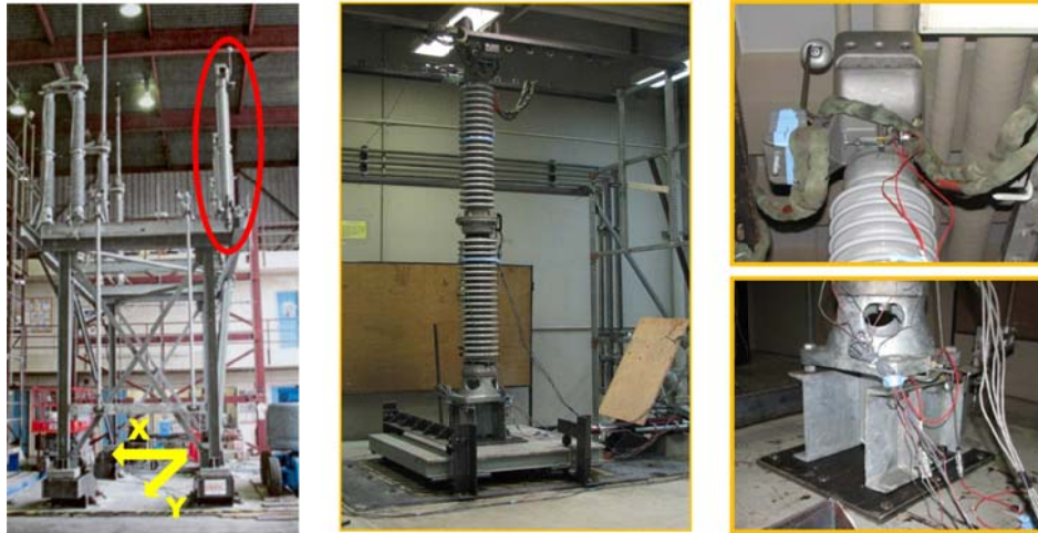
Figure 4.1 As-installed 230-kV disconnect switch mounted on the PEER shaking table during a seismic qualification test in 2008 (left), substructured single insulator post setup (middle) and close-up views of single insulator base connection and top live parts (right).
