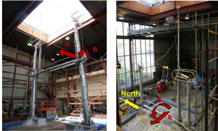
Figure 3.1 Test setup for 550-kV as-installed switch test (left) and substructured switch without support structure (right) showing signals generated from the as-installed test and applied to the substructured test.
