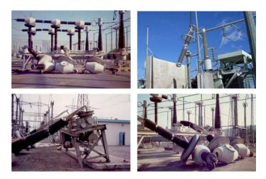
Figure 1.1 Failure examples of porcelain insulators after earthquakes (Fujisaki, 2009).
