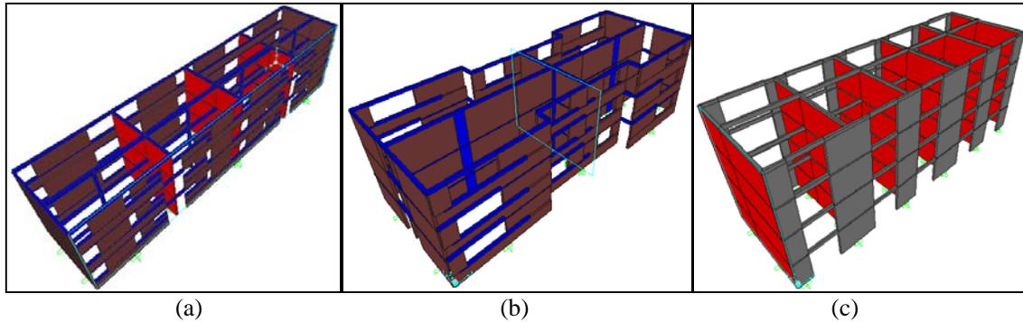
**Figure 4.** (a) Model of building type B1, (b) Model of building type B3 and (c) Model of building type C1
