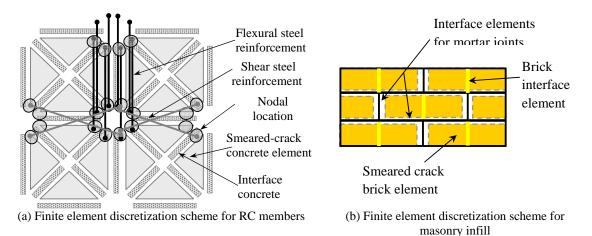
Figure 2. Finite element modeling schemes.
