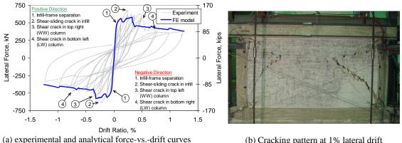
ental and analytical force-vs.-drift curves (b) Cracking pattern at 1% lateral drift **Figure 3.** Finite element modeling schemes.
