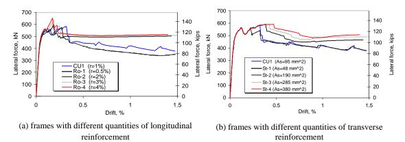
Figure 6. Effect of (a) longitudinal, (b) transverse column reinforcement on the load-vs.-drift curves of frames.
