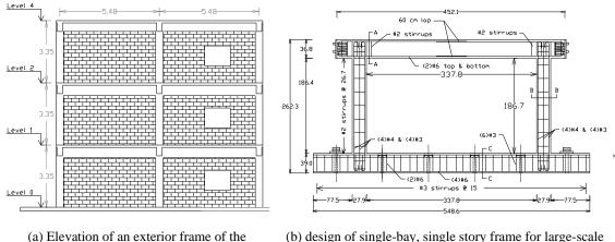
(a) Elevation of an exterior frame of the prototype (dimensions in m).
