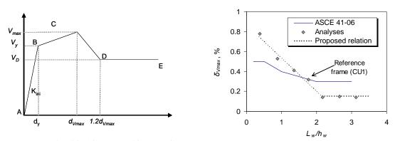
(a) Proposed simplified force-vs.-drift curves for RC frames with solid panels.
