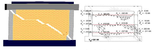
(a) failure pattern of numerical model at 1% drift (b) force distribution along five cross sections at the instant of peak load Figure 4. Results obtained from the analytical model.
