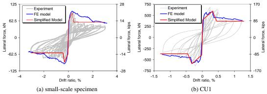
Figure 9. Comparison of simplified curves with experimental results.
