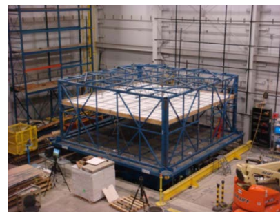
Figure 2.1. New test frame: 6.3 \text{ m} \times 16.5 \text{ m} large test set up (left) and 6.3 \text{ m} \times 6.3 \text{ m} small test set up (right)
