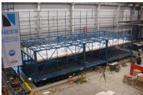
Figure 2.1. New test frame: 6.3 \text{ m} \times 16.5 \text{ m} large test set up (left) and 6.3 \text{ m} \times 6.3 \text{ m} small test set up (right)
