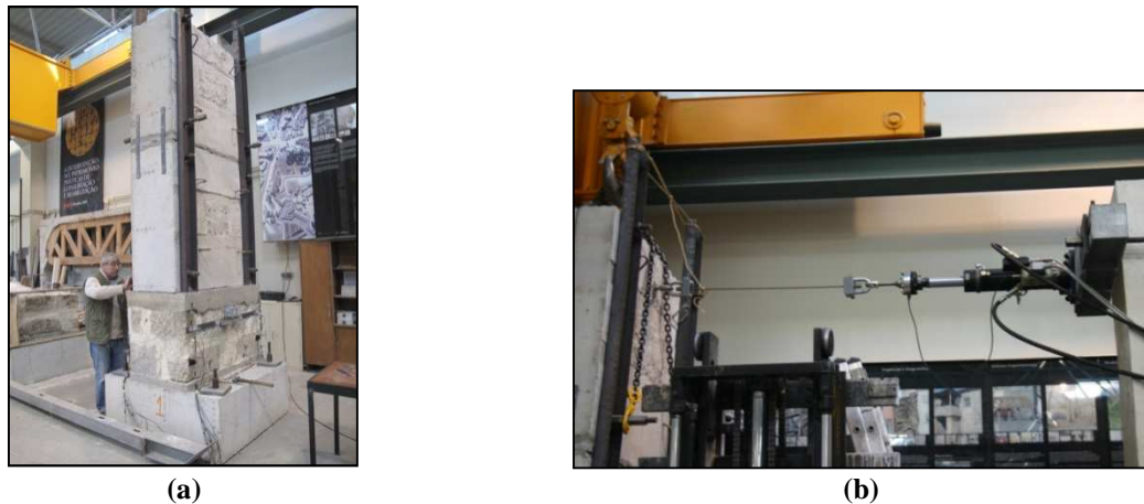
Figure 3.1: Specimen test under free rocking motion: a) test apparatus; b) pullout scheme
