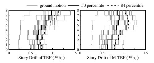
Figure 4.1. Comparison of storey drift demand between the TBF and M-TBF systems.
