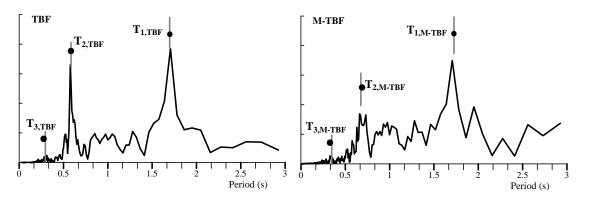
Figure 4.5. Power spectral of roof drift under Hector Mines Joshua Tree, 1999
