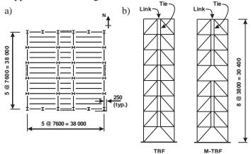
Figure 2.1 Building structure studied: a) Floor plan; b) Elevation of the 8-storey TBF and M-TBF frames.
