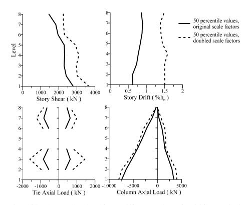
Figure 4.6. Comparison of the 50 percentile values of storey drifts, storey shears, tie axial forces and column axial forces under ground motion set with different scale factors
