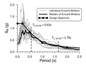
Figure 3.1 Design spectrum and 5% damped absolute acceleration spectra of the ground motion records.
