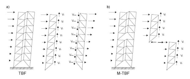
Figure 2.2. Design of the links in: a) TBF system; b) M-TBF system.
