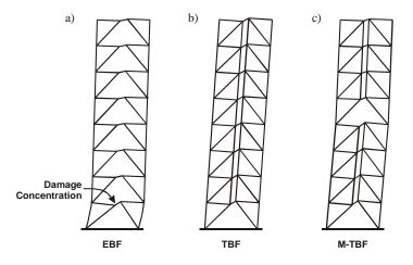
Figure 1.1 EBF systems: a) EBF; b) TBF, and c) proposed M-TBF.
