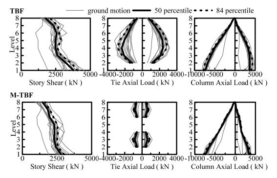
Figure 4.3. Comparison of storey shear, tie and column axial forces between the TBF and M-TBF systems.
