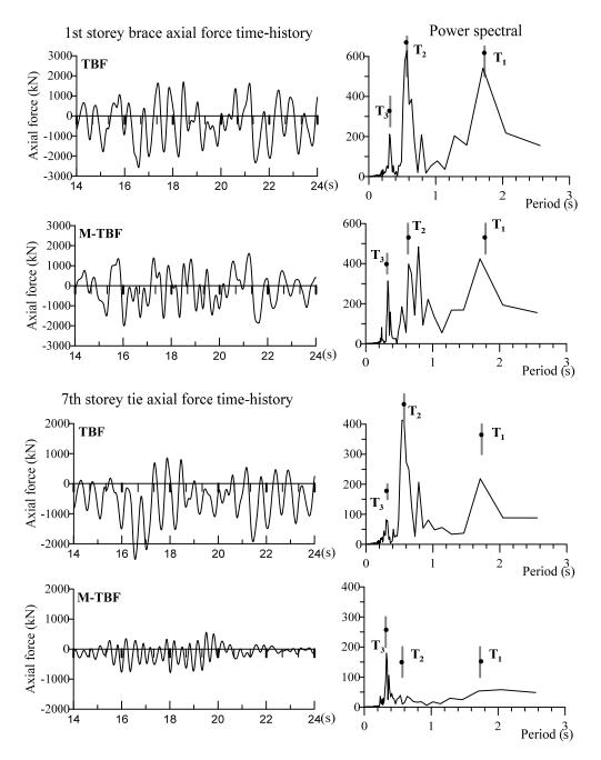
Figure 4.4. Comparison of brace and tie responses in time domain and frequency domain under Hector Mines, Joshua Tree, 1999
