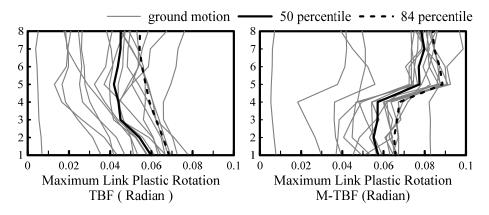
Figure 4.2. Comparison of link plastic rotation between the TBF and M-TBF systems.
