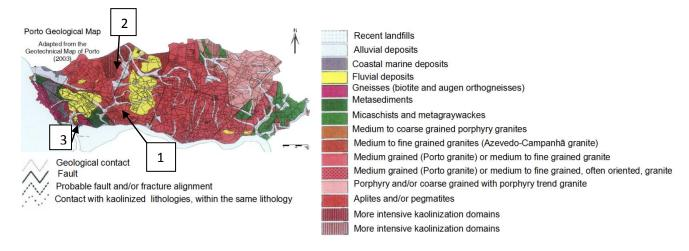
Figure 2. The Geotechnical Map of Porto along with the locations of three of the seismic dispersive surface wave tests. (Adapted from Almeida and Begonha, 2008)
