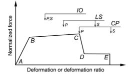
Figure 4.1- Behavior and performance limits in a typical hinge (FEMA 356, 2000)
