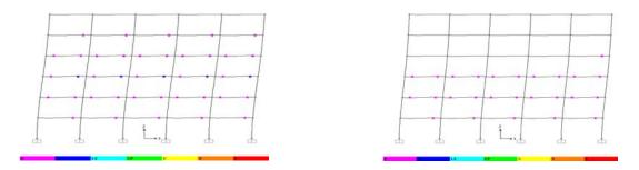
(a) x direction (b) y direction **Figure 4.2.** Status of plastic hinges of the 6 storey structure at the end of the pushover analysis under the triangular loading
