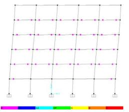
(a) x direction (b) y direction **Figure 5.1.** Status of plastic hinges of the 6 storey structure at the end of the pushover analysis under the triangular loading
