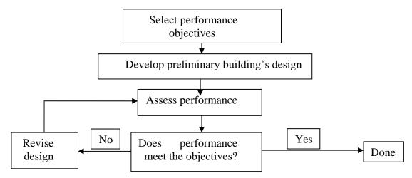
Figure1.1 Performance-based design flowchart (FEMA 445-B, 2006)
