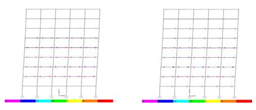
(a) x direction (b) y direction **Figure 4.5.** Status of plastic hinges of the 9 storey structure at the end of the pushover analysis under the rectangular loading
