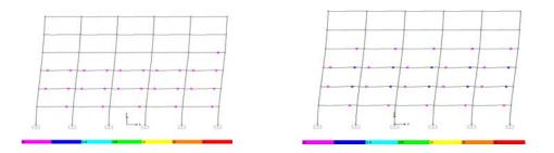
(a) x direction (b) y direction **Figure 4.3.** Status of plastic hinges of the 6 storey structure at the end of the pushover analysis under the rectangular loading
