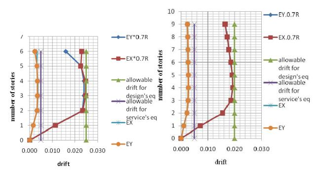
Figure 3.1- Drift angle of the structures against the service and the design level earthquakes
