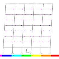
(a) x direction (b) y direction **Figure 4.4.** Status of plastic hinges of the 9 storey structure at the end of the pushover analysis under the triangular loading
