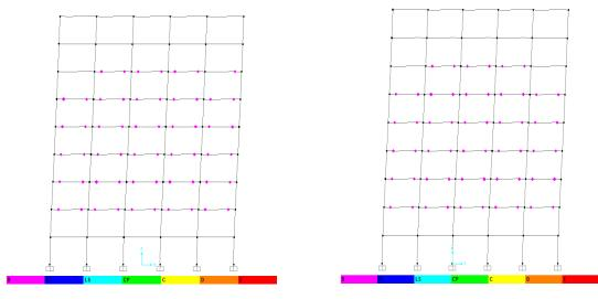
Figure 5.5. Status of plastic hinges of the 9 storey structure at the end of the pushover analysis under the triangular loading
