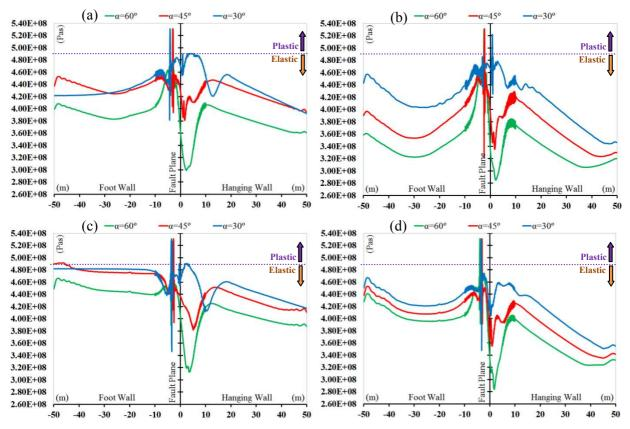
**Figure 2.5.** Influence of Fault-Pipe Intersection Angle on Stress Response of Pipelines Buried in: (a) Soil CSO (b) Soil CST (c) Soil GLO (d) Soil GDE (*D*/*t*=96, Crown Edge of Pipeline)
