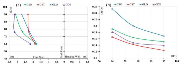
**Figure 2.3.** Influence of the Pipe Wall Thickness on (a) Failure Position of Elements Located at Crown Edge of Pipeline (b) Failure Fault Plane displacement to Diameter Ratio ( $\Delta f/D$ ) With Respect to D/t. ( $\alpha = 45^{\circ}$ )
