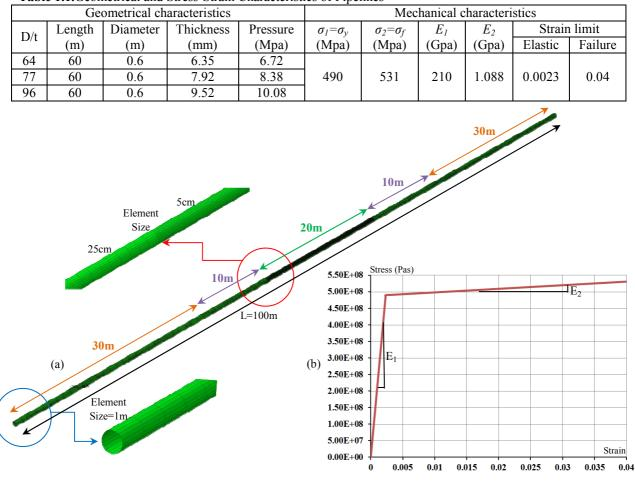
Table 1.1.Geometrical and Stress-Strain Characteristics of Pipelines
