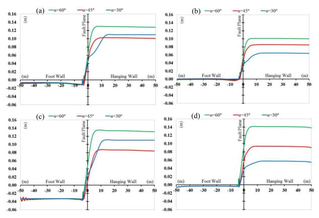
**Figure 2.4.** Influence of Fault-Pipe Intersection Angle on Peak Failure Displacement of Pipelines Buried in: (a) Soil CSO (b) Soil CST (c) Soil GLO (d) Soil GDE (*D/t=96*, Crown Edge of the Pipelines)
