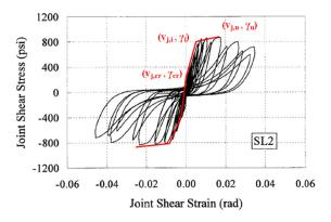
Figure 3.1. Critical Points of the Joint Model Presented on Specimen SL2 by Shin and LaFave (2004-a)
