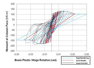
Figure 4.3. Beam Moment at Column Face versus Beam Plastic Hinge Rotation Response of Specimen 2-S by Burak and Wight (2008) with and without the joint model
