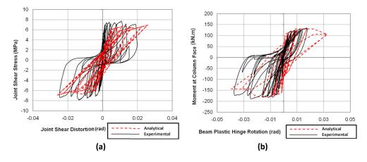
Figure 4.2. (a) Joint Shear Stress versus Joint Shear Distortion Response of Specimen 2-S by Burak and Wight (2008)
