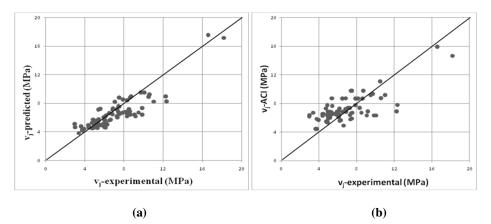
**Figure 3.2.** (a) Predicted versus experimental joint shear strength (b) ACI 352-02 recommended versus experimental joint shear strength
