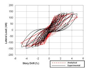
Figure 4.1. Lateral Load versus Story Drift Response of Specimen 2-S by Burak and Wight (2008)
