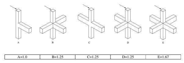
Figure 2.1. Joint Types and Joint Type Index (JT) Values for Computations in SI Units
