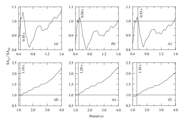
**Figure 5.4:** Ratio of mean acceleration spectrum of the late arriving pulse motions (SA<sub>LP</sub>) to mean acceleration spectrum of the early arriving pulse motions (SA<sub>EP</sub>) versus period for motions (a) scaled at 0.45 s, (b) scaled at 0.50 s, (c) scaled at 0.55 s, (d) scaled at 1.10 s, (e) scaled at 1.20 s, and (f) scaled at 1.30 s.
