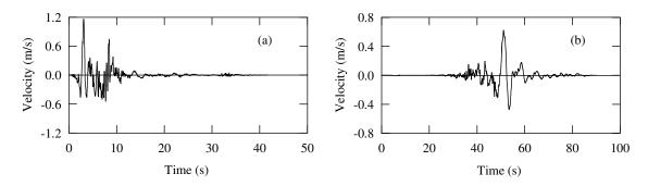
**Figure 1.1:** Velocity time histories of ground motions recorded at (a) Pacoima Dam (upper left abutment) recording station during the 1971 San Fernando earthquake (NGA no. 77) and (b) TCU029 recording station during the 1999 Chi-Chi earthquake (NGA no. 1476).
