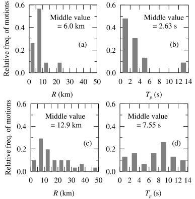
Figure 2.5: distribution of motions with the *R* and  $T_p$  for 2.5(a)-2.5(b) for the early arriving and 2.5(c)-2.5(d) the late arriving pulse motions.
