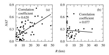
Figure 2.2: NAT versus R plot for motions originated from (a) dip-slip faults and (b) strike-slip faults.
