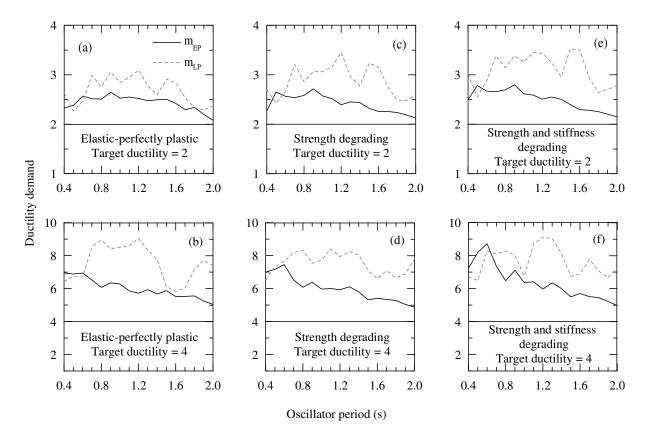
**Figure 5.1:** Mean ductility demand versus oscillator period for the early arriving pulse (m<sub>EP</sub>) and the late arriving pulse (m<sub>LP</sub>) motions for (a, b) elastic-perfectly plastic oscillators, (c, d) strength degrading oscillators, and (e, f) strength and stiffness degrading oscillators for target ductility 2 and 4.
