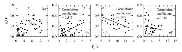
**Figure 2.3:** *NAT* versus  $T_p$  plot for motions originated from (a) dip-slip faults, (b) dip-slip faults and having pulse period less than 6.5 s, (c) dip-slip faults and having pulse period more than 6.0 s, and (d) strike-slip faults.
