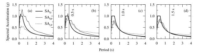
Figure 4.1: Design acceleration spectrum  $(SA_D)$  and mean acceleration spectrum of the early arriving pulse  $(SA_{EP})$  and the late arriving pulse  $(SA_{LP})$  motions (a) unscaled, (b) scaled at 0.5 s, (c) scaled at 1.0 s, and (d) scaled at 1.5 s.
