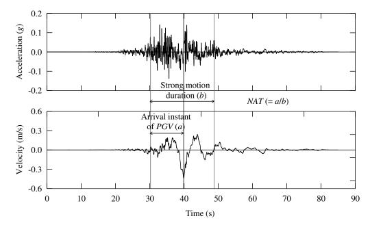
**Figure 2.1:** Illustration of *NAT* using acceleration and velocity time-histories of ground motion recorded at TCU046 recording station during the 1999 Chi-Chi earthquake (NGA no. 1486).
