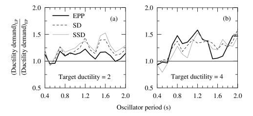
**Figure 5.3:** Ratio of mean ductility demand for the late arriving pulse motions to mean ductility demand for the early arriving pulse motions versus oscillator period for elastic-perfectly plastic (EPP), strength degrading (SD), and strength and stiffness degrading (SSD) oscillators for (a) target ductility 2 and (b) target ductility 4.
