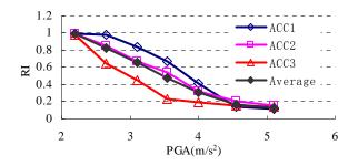
Figure 4.3. Reparability index curve of the building
