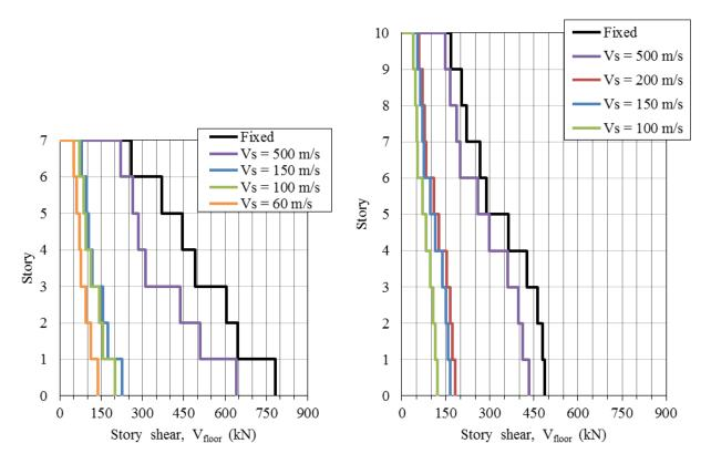
Figure 6. Maximum story shear for buildings due to Victoria earthquake (PGA = 0.3g)
