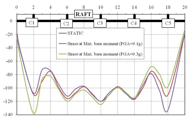
Figure 9. Distribution of contact stresses (kPa) for the 10-story building due to different load cases- Kobe earthquake ( $V_s$ =150 m/sec)
