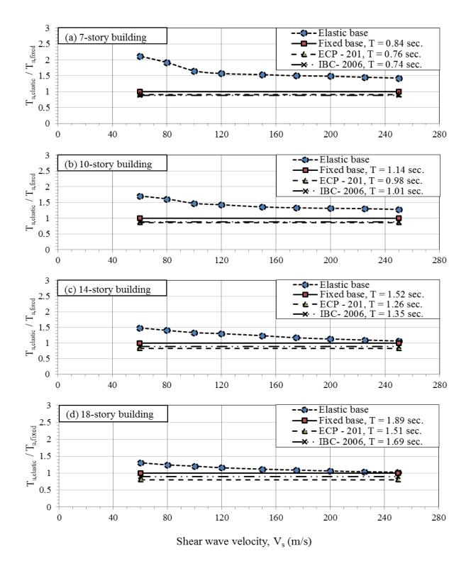
**Figure 3.** Effect of soil shear modulus (V<sub>s</sub>) on fundamental period of buildings with variable heights: a)7-story; b) 10-story; c) 14-story; d) 18-story
