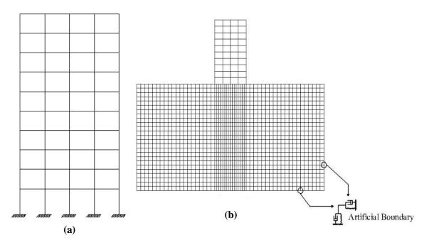
Figure 1. Ten-story building models: (a) Fixed foundation; (b) Elastic foundation
