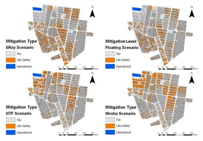
**Figure 2:** Distribution of mitigation alternative in the pilot area for South Ray Fault scenario (2.a Up-left), Floating scenario (2.b Up-right), North Tehran Fault scenario (2.c Bottom-left) and Mosha fault scenario (2.d Bottom-right)
