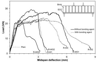
**Figure 2.8.** Flexural response of the masonry beams
