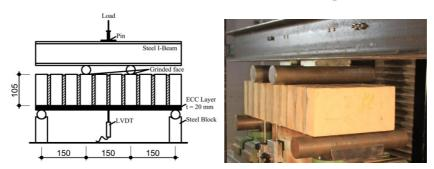
Figure 2.7. (a) Four-point bending test schematic view and dimensions (b) test setup and instrumentation
