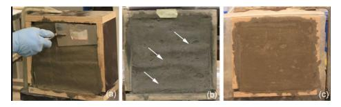
**Figure 2.3.** (a) Applying ECC layer (b) ruffled surface of hardened ECC (c) flat surface of hardened ECC after adjusting water and superplasticizer
