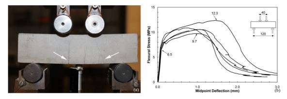
Figure 2.2. (a) Four point bending test setup and multiple cracking of ECC (b) ECC flexural Stress-deflection behavior
