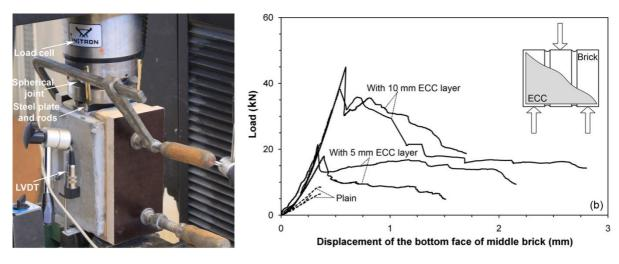
Figure 2.10. (a) Triplet test setup (b) Load-displacement curves obtained from the triplet tests
