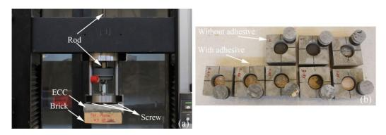
Figure 2.4. (a) Test setup (b) the test specimens after failure in tension
