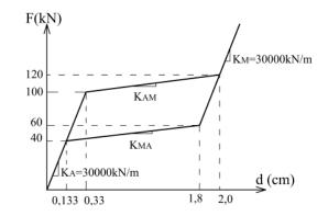
Figure 2.3. Force – deformation diagram for the designed damper
