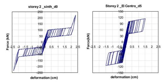
Figure 4.5 Force-deformation diagrams for the dampers at second storey of frame R<sub>2</sub>
