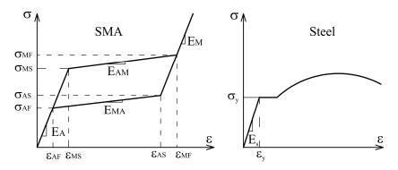
Figure 2.2. Stress strain diagrams for damper main parts
