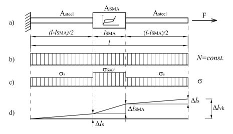
Figure 2.1. State of stress and deformation at axially loaded hybrid damper made with serial connected elements
