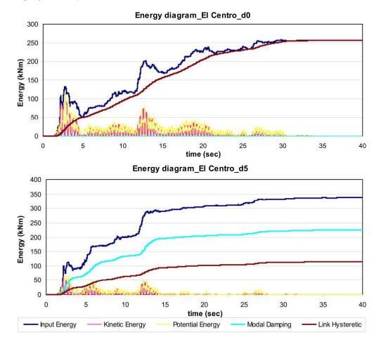
Figure 4.6 Energy diagrams for El Centro time history analysis with 0 and 5% modal damping
