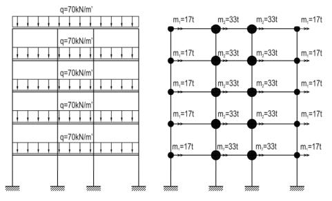
Figure 4.2. Distribution of loads and mass at the analyzed frames
