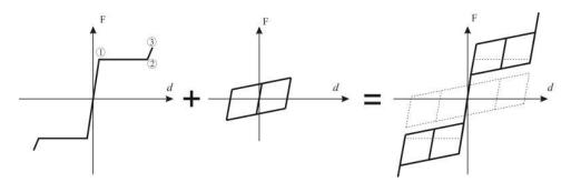
Figure 3.1. Schematic representation of the element behaviour obtained by parallel connection of linear elastic and Wen plastic model
