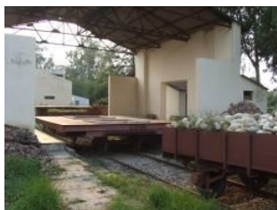
Figure 3.2. Shock table test facility showing the shock table and loaded end wagons
