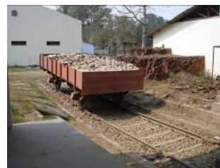
Figure 3.2. Shock table test facility showing the shock table and loaded end wagons
