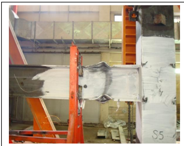
Figure 14. Specimen LF30-T at the end of the test.
