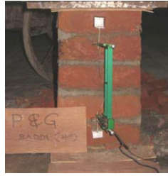
Figure 9. Five brick masonry prisms compression testing.
