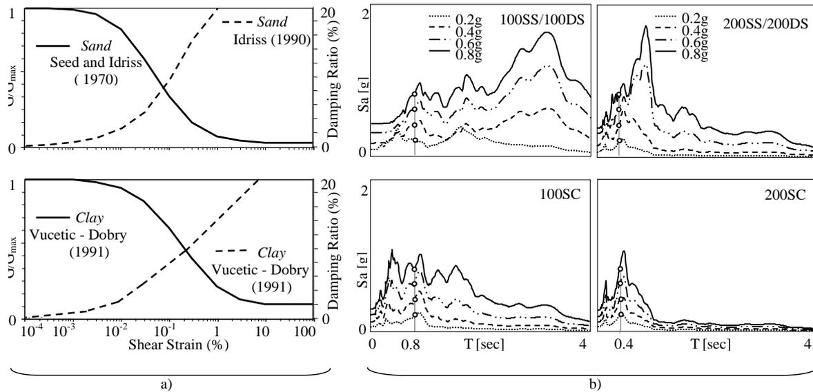
**Figure 4.** a) Variation of shear modulus and damping ratio with shear strain; b) Imperial Valley earthquake: acceleration response spectra of the ground surface motion
