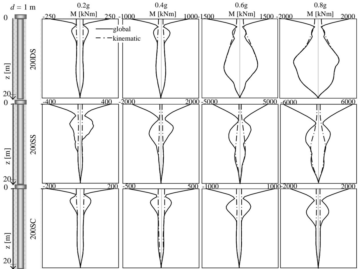
**Figure 8.** Envelope of bending moments obtained performing IDAs analyses for  $V_s = 200$  m/s.
