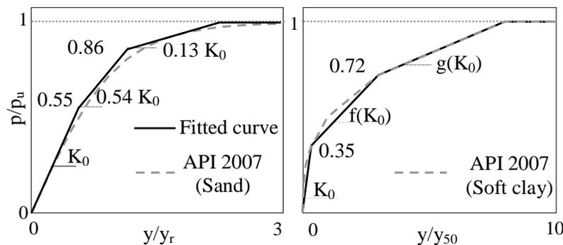
Figure 2. Typical 4-segment curve fit to the hyperbolic curve
