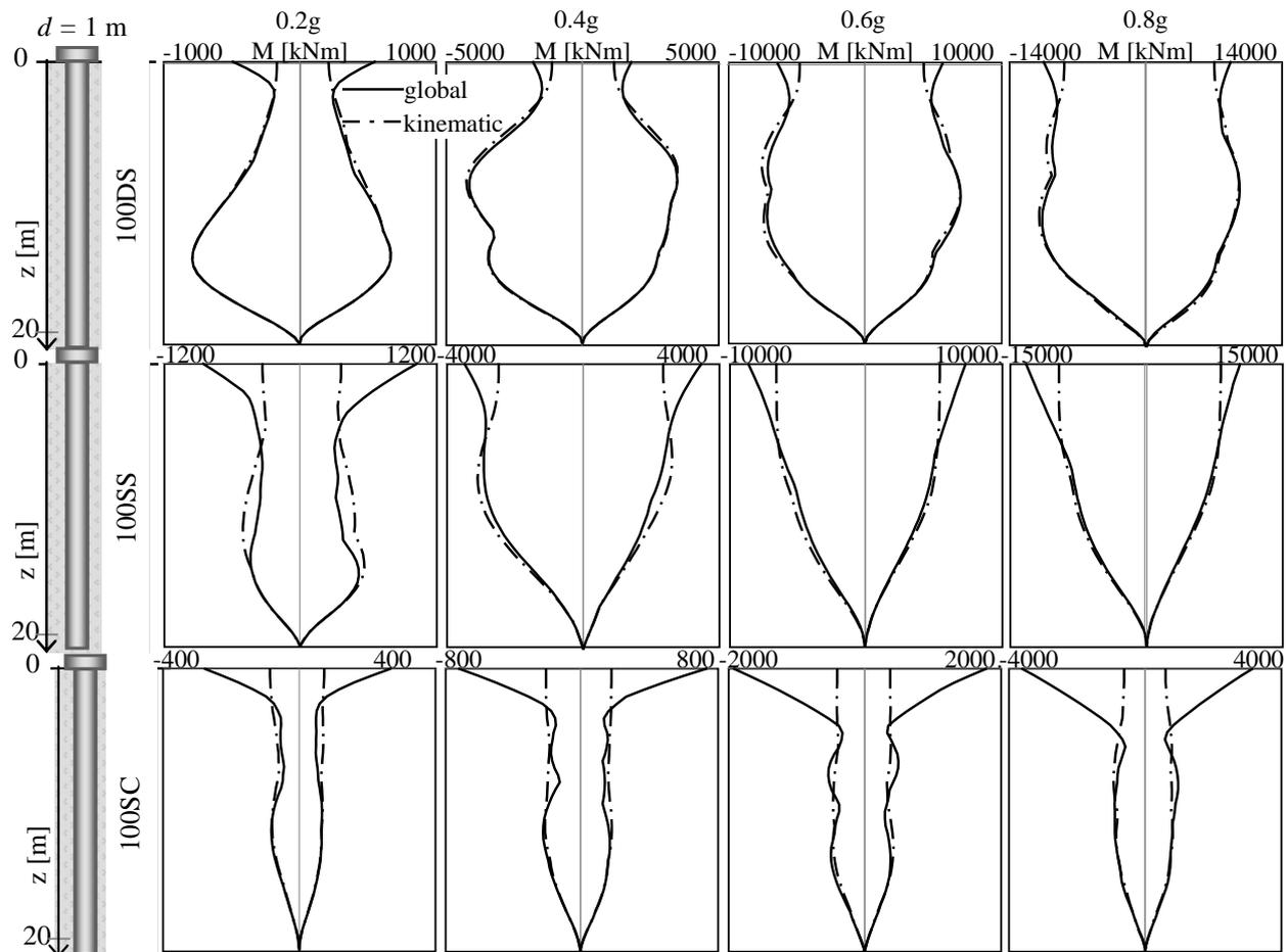
**Figure 7.** Envelope of bending moments obtained performing IDAs analyses for  $V_s = 100$  m/s.
