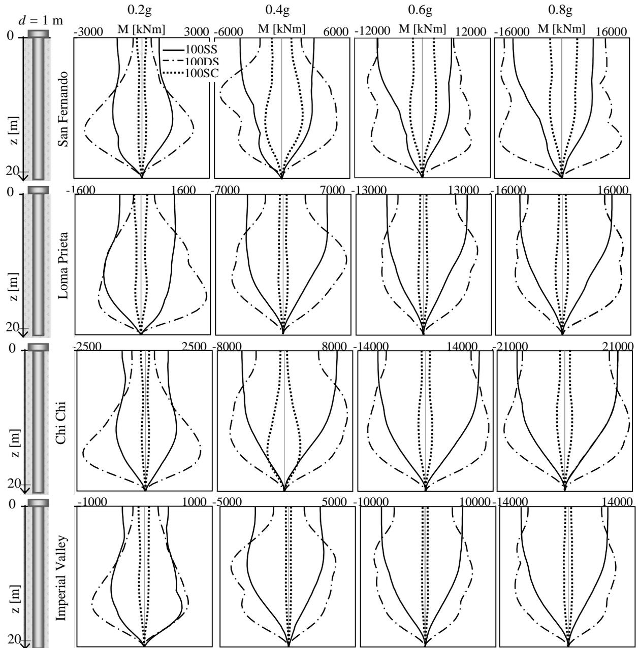
**Figure 5.** Envelope of bending moments obtained performing IDAs for soil profiles with  $V_s = 100$  m/s.
