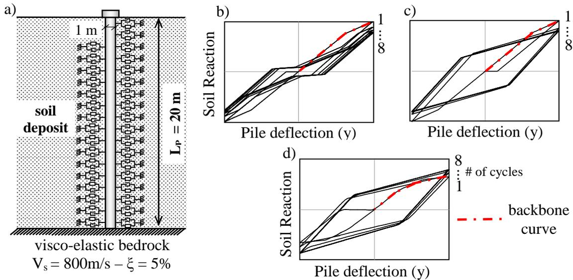
**Figure 1.** a) Soil profile and BNWF model; Hysteretic curves: b) S-shaped hysteresis curve; c) oval-shaped hysteresis curve and d) hardening response
