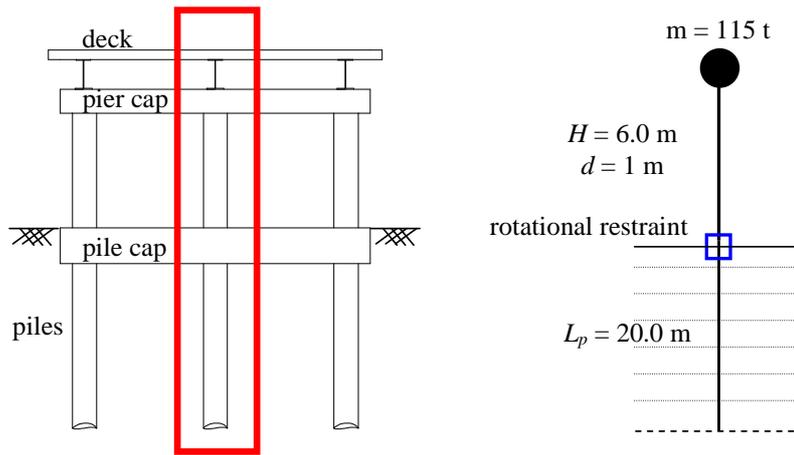
**Figure 6.** a) Multi-column bent; b) Schematic illustration of the analysed problem.
