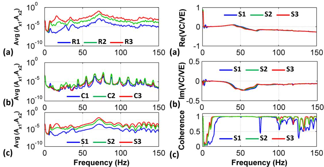
**Figure 3.** Averaged horizontal PSD  $((m/s^2 \text{rms})^2/\text{Hz})$  for VE excitation of pile U in unimproved soil. (a) Random, (b) Chaotic impulse, (c) Swept-sine loading at intensity levels 1, 2, and 3.
