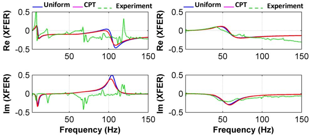
**Figure 9.** Effect of soil modulus variation on the transfer function of the system and comparison with U-HC-S2 and U-VC-S2. (a) Horizontal transfer function at  $A_{x2}$  in HC test, (b) Vertical transfer function at  $A_{z2}$  in VC test.
