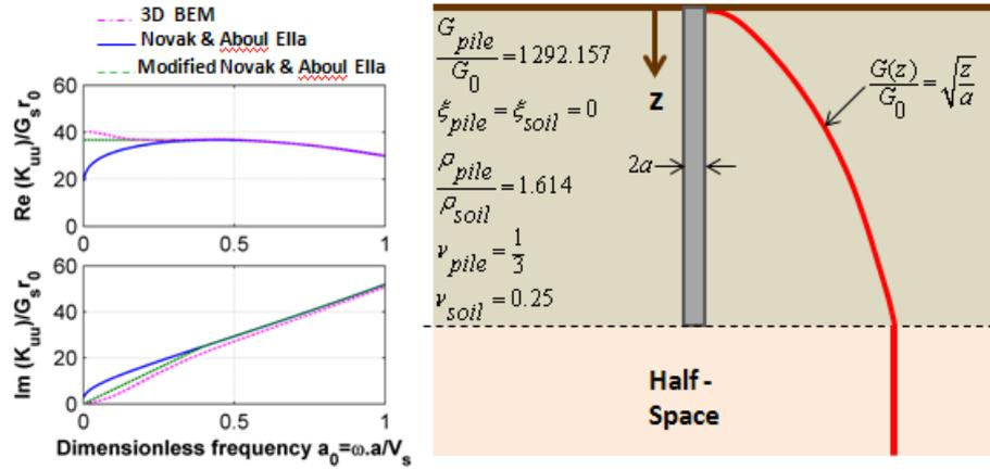
**Figure 7.** Verification of the MATLAB program written for the approximate solution by comparison against the rigorous 3D boundary element program BEASSI. Horizontal impedance  $K_{uu}$  is shown.
