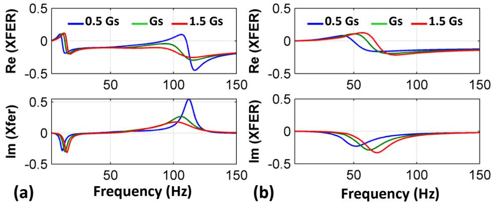
**Figure 10.** Effect of soil modulus value on the transfer function of the system. (a) Horizontal transfer function at  $A_{x2}$  in HC test, (b) Vertical transfer function at  $A_{z2}$  in VC test.
