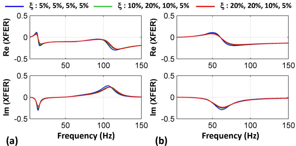
**Figure 11.** Effect of soil damping on the transfer function of the system. Damping ratios shown in the legend correspond to the four soil layers, from top to bottom. (a) Horizontal transfer function at  $A_{x2}$  in HC test, (b) Vertical transfer function at  $A_{z2}$  in VC test.
