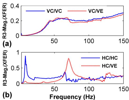
**Figure 5.** Comparison of VE test to combination of VC and HC tests for random excitation in unimproved soil. (a) VC response from VC and VE tests, (b) HC response from HC and VE tests.
