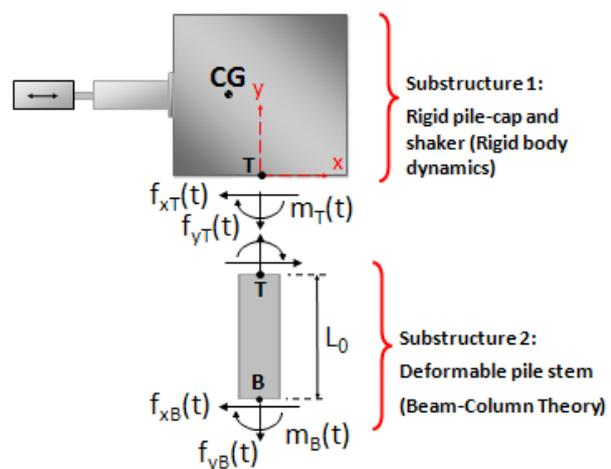
**Figure 6.** Substructures and interfacial forces used in transfer function formulation.
