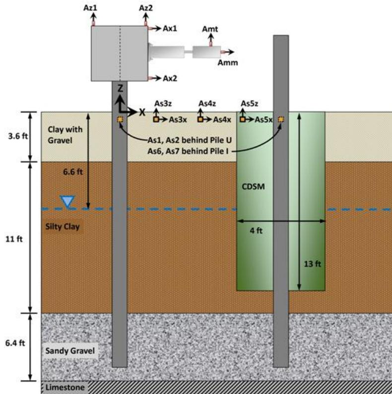
**Figure 1.** Soil profile and orientation and notation for accelerometers on shaker and pile cap (shaker shown in HC test position on pile U).
