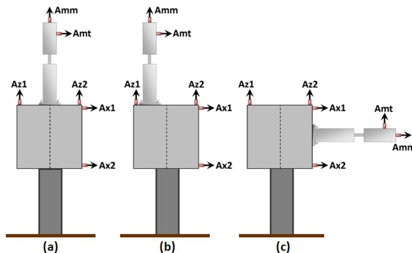
**Figure 2.** Inertial shaker configurations for the three test types; (a) VC test, (b) VE test, (c) HC test.
