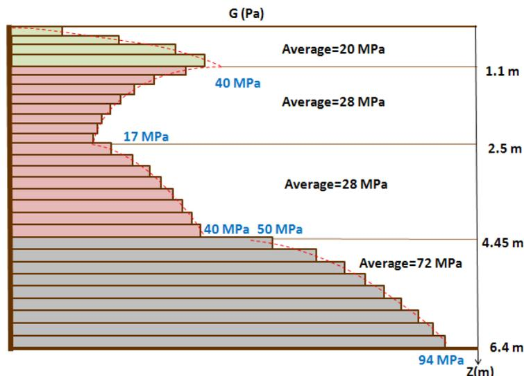
**Figure 8.** Shear modulus profile from CPT test data
