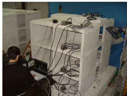
Figure 3.4. 3D view of test setup for forced vibrations of specimens.
