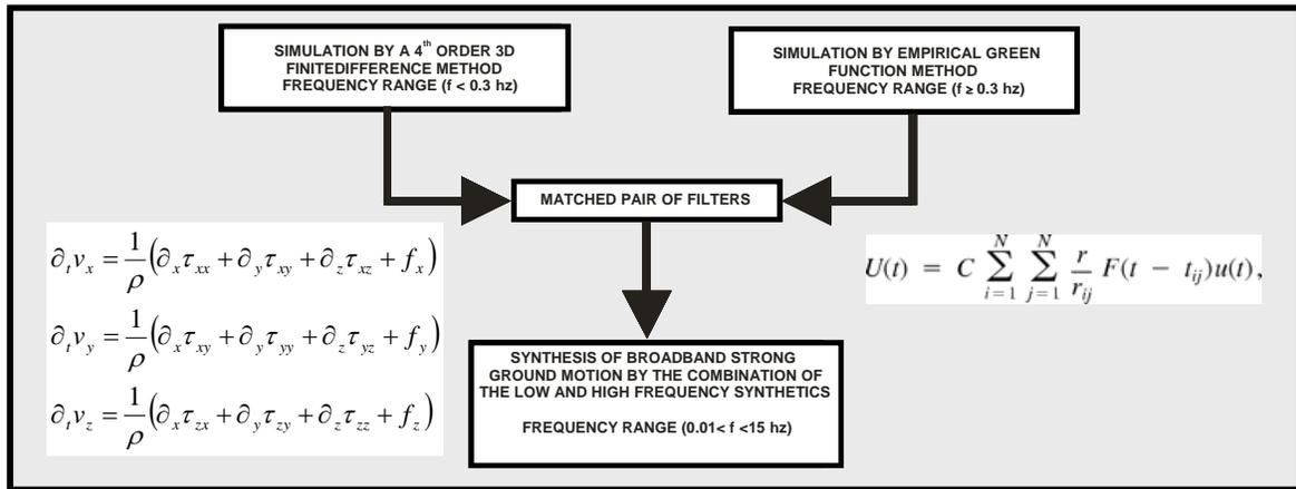
**Figure 1.** Hybrid procedure combining long period and high frequency simulations (Chavez et al., 2011)
