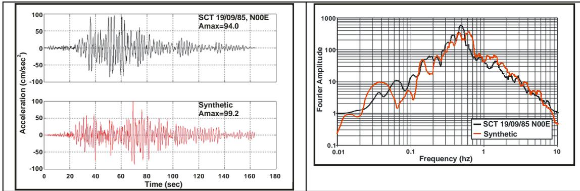
**Figure 3.** Observed and synthetic accelerograms and their corresponding Fourier amplitude spectra in the N-S direction at station SCT (Mexico City) for the 19 September 1985 Michoacan earthquake
