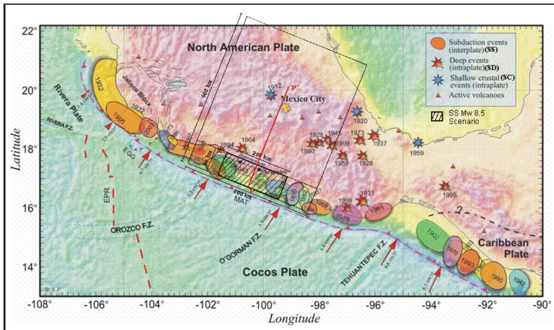
**Figure 4.** 3D volume ( $500 \times 600 \times 124 \text{ km}^3$ ) utilized in the 3D Finite Differences Modeling of the Mw 8.5 thrust surficial subduction Guerrero gap earthquake scenarios (Modified, Pacheco and Kostoglodov, 1999)
