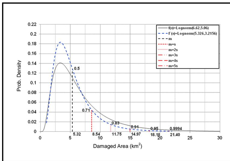
**Figure 11.** Lognormal probability density functions of damaged areas in Mexico City for the Mw 8.5 scenario earthquakes. The dashed curve correspond to the truncated distribution which includes the damaged areas for different probabilities of exceedances
