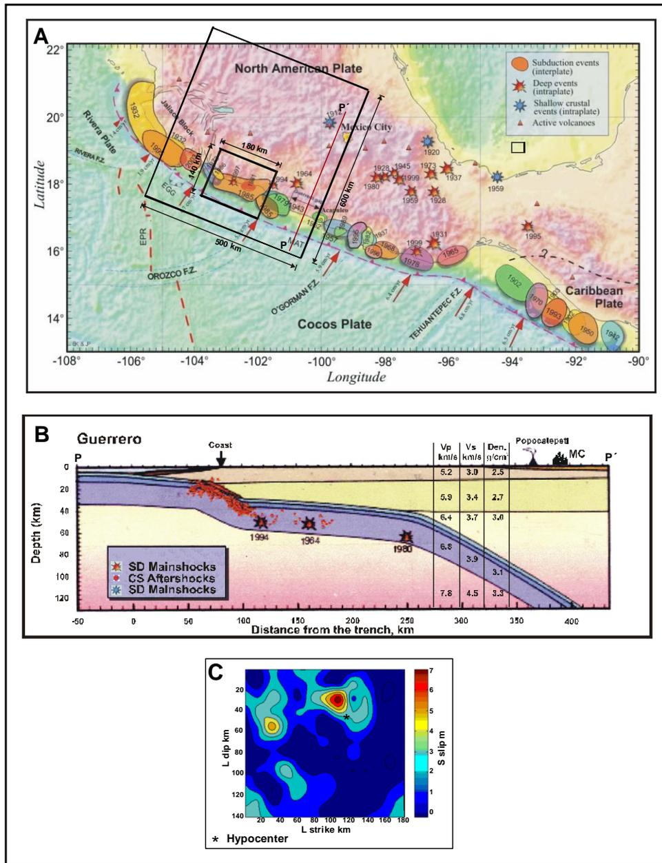
**Figure 2.** A) Inner rectangle is the rupture area of the 19 September 1985 Ms 8.1 earthquake on the surface projection of the 500x600x124 km<sup>3</sup> earth crust volume 3D discretization; B) profile P-P'; C) Kinematic slip distribution of the rupture of the 1985 earthquake. (A and B, Modified, Pacheco and Kostoglodov, 1999, and C, Modified, Mendoza and Hartzell, 1989)
