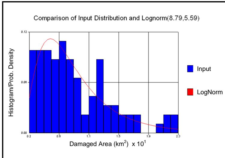
**Figure 10.** Histogram and fitted Lognormal probability density distribution of damaged areas in Mexico City for the Mw 8.5 earthquake scenarios
