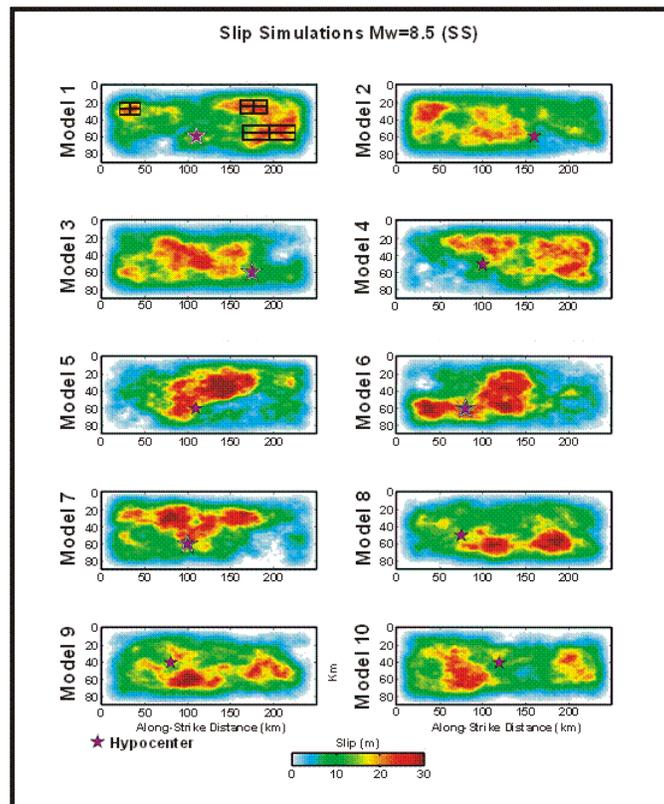
**Figure 5.** Fractal slip simulations (based on Mai and Beroza, 2002) of the finite seismic sources used in the hybrid modeling of the Mw 8.5 extreme Thrust Subduction Surficial (TSS) earthquake scenarios. The rectangles in model 1 are an example of the finite sources used for the Empirical Green Functions simulations
