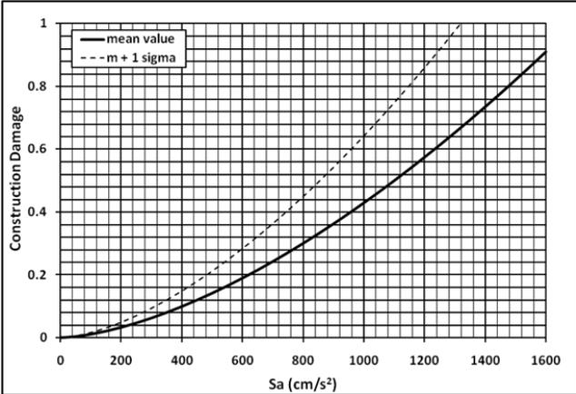
**Figure 9.** Vulnerability functions of Mexico City construction stock of 1 to 3 levels used for the estimation of the probability density of exceedances of the economical consequences, PEDEC's, for the Mw 8.5 earthquake scenarios (Modified, Ordaz et al., 1994)
