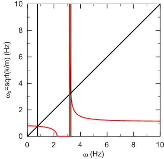
**Figure 1.** Schematic of bisector solution for identifying resonant frequency of a two DOF undamped system
