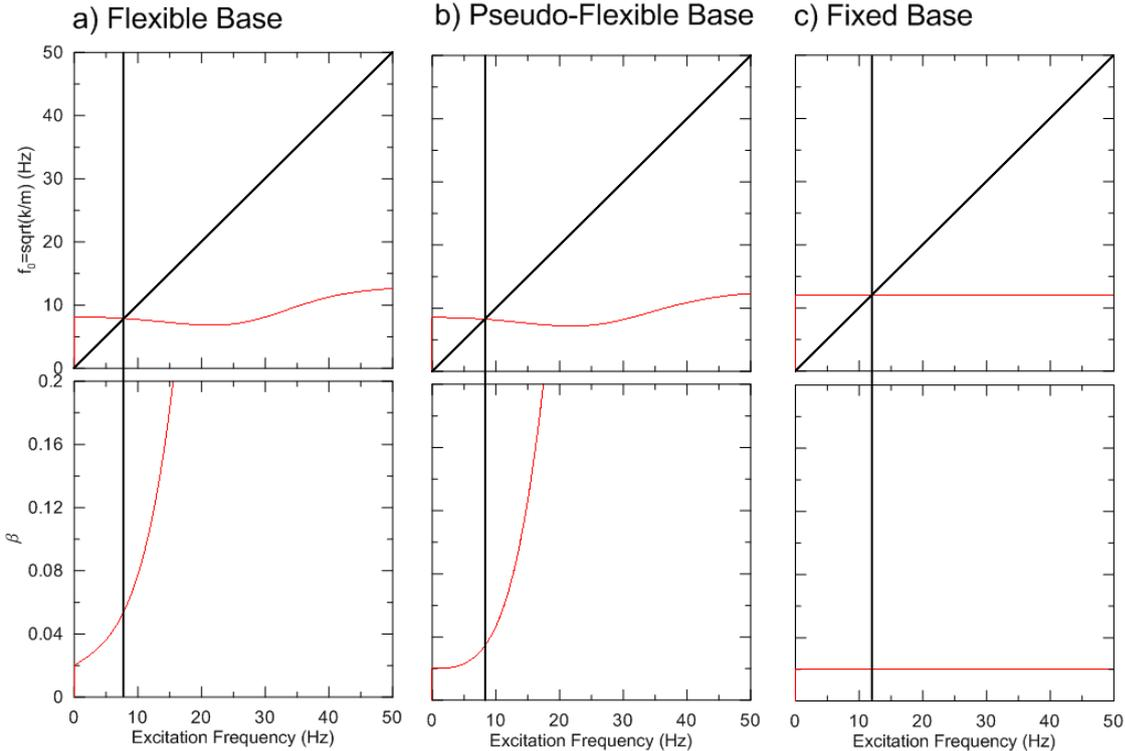
**Figure 3.** Bisector identification of frequency and damping for forced vibration (FV) loading of a SDOF modeled structure for (a) flexible base, (b) pseudo-flexible base and (c) fixed base conditions.
