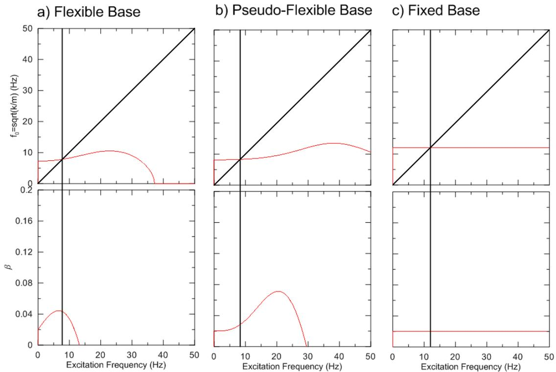
**Figure 4.** Bisector identification of frequency and damping for earthquake (EQ) loading of a SDOF modeled structure for: (a) flexible base, (b) pseudo-flexible base and (c) fixed base conditions.
