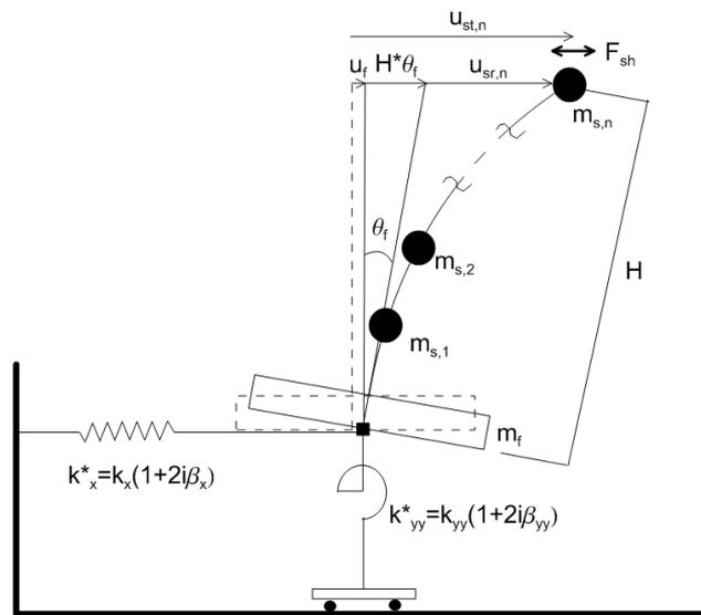
**Figure 2.** A simple SSI System subjected to forced vibration at roof node
