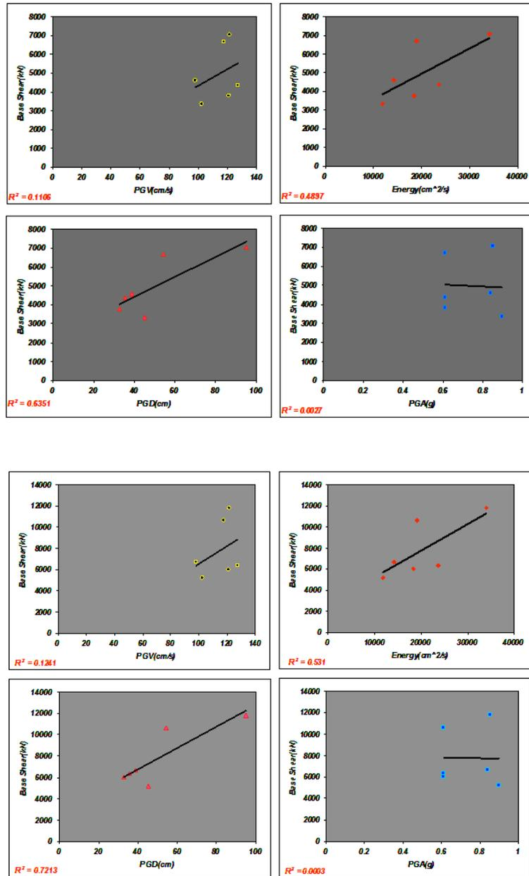
**Figure 3.2.** Variation of the Maximum Dynamic Base Shear versus the Near-Field Ground Motion Parameters in the “IO” Building, 5-Story(Top), 8-Story(Bottom) [4]
