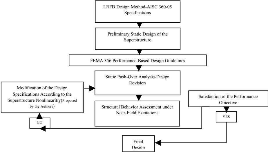
Figure 2.1. Performance-Based Design Steps of the Isolated Buildings[4]
