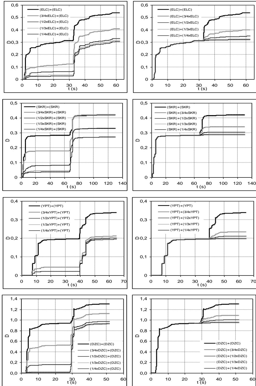
**Figure 3.5.** Damage curves for a SDOF subjected to the synthetic acceleration histories comprising El Centro 1940, NS component and its various amplitude **a)** El Centro 1940, NS comp., **b)** Aug. 17, 1999 Marmara Earthquake, Sakarya Station, EW comp., **c)** Aug. 17, 1999 Marmara Earthquake, Yarımca Petrochemical Complex Station, NS comp., **d)** Nov. 12, 1999 Düzce Earthquake, Düzce Station, NS comp.
