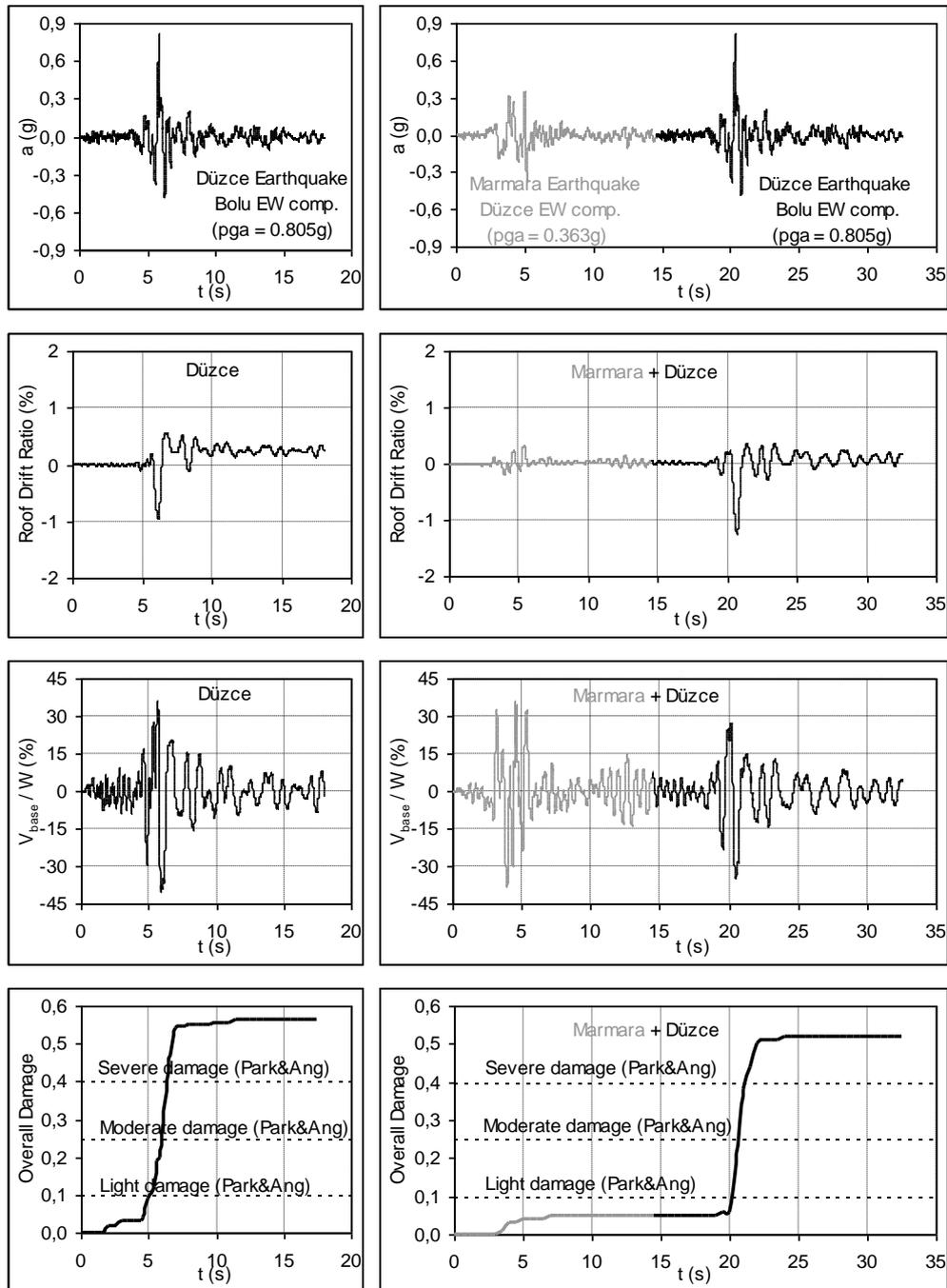
**Figure 4.2.** Ground acceleration histories, roof drift ratio variations, base shear ratio variations and damage curves for transverse (east-west) direction of the building
