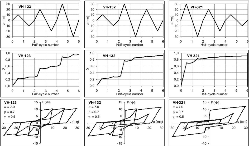
**Figure 3.2.** Variable-amplitude loading histories, damage curves and force-displacement relationships
