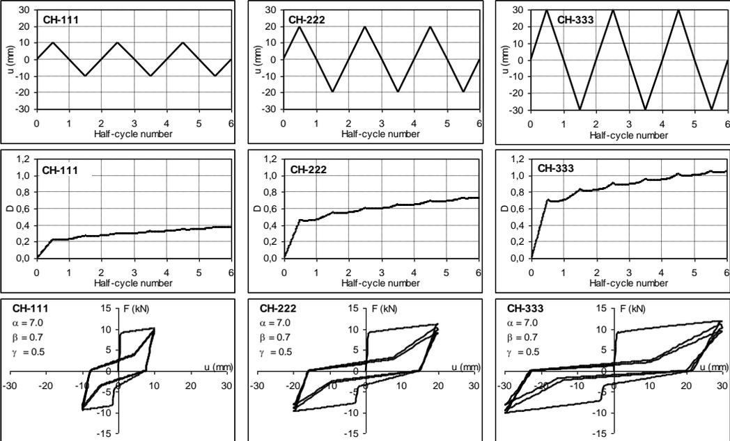
**Figure 3.1.** Constant amplitude loading histories, damage curves and force-displacement relationships
