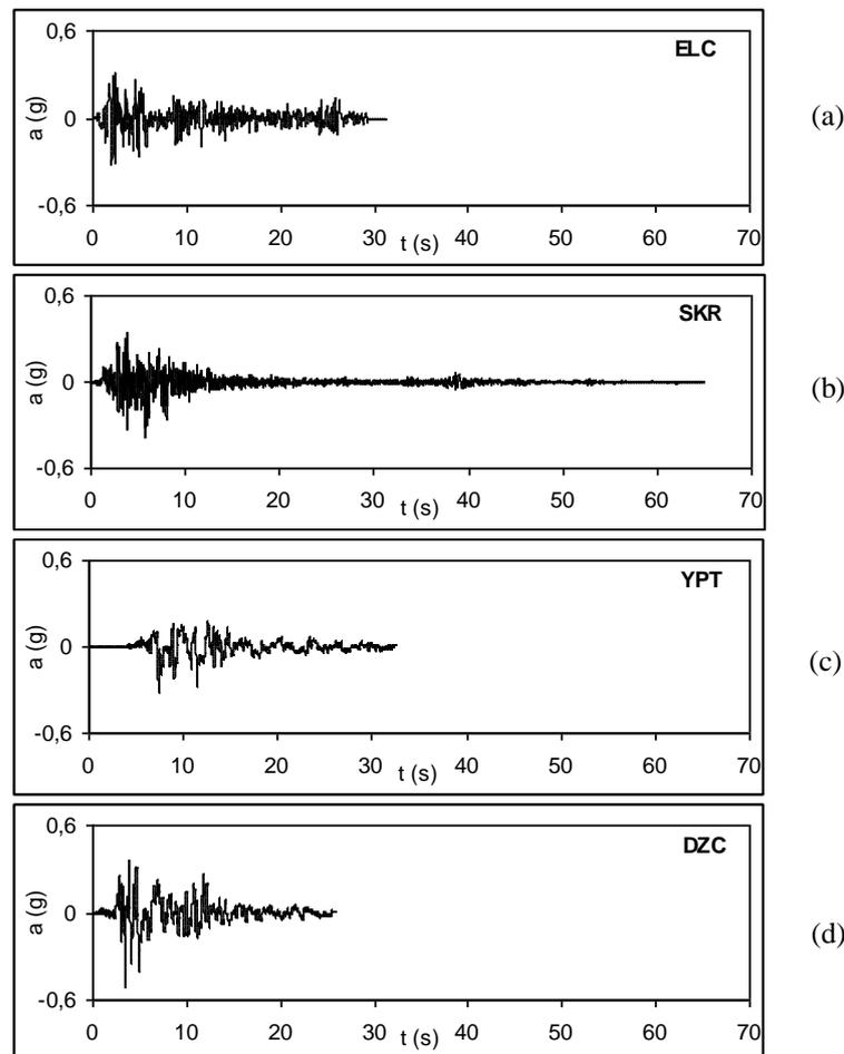
**Figure 3.4.** The ground motions used in this study. **a)** El Centro 1940, NS comp., **b)** Aug. 17, 1999 Marmara Earthquake, Sakarya Station, EW comp., **c)** Aug. 17, 1999 Marmara Earthquake, Yarımca Petrochemical Complex Station, NS comp., **d)** Nov. 12, 1999 Düzce Earthquake, Düzce Station, NS comp.
