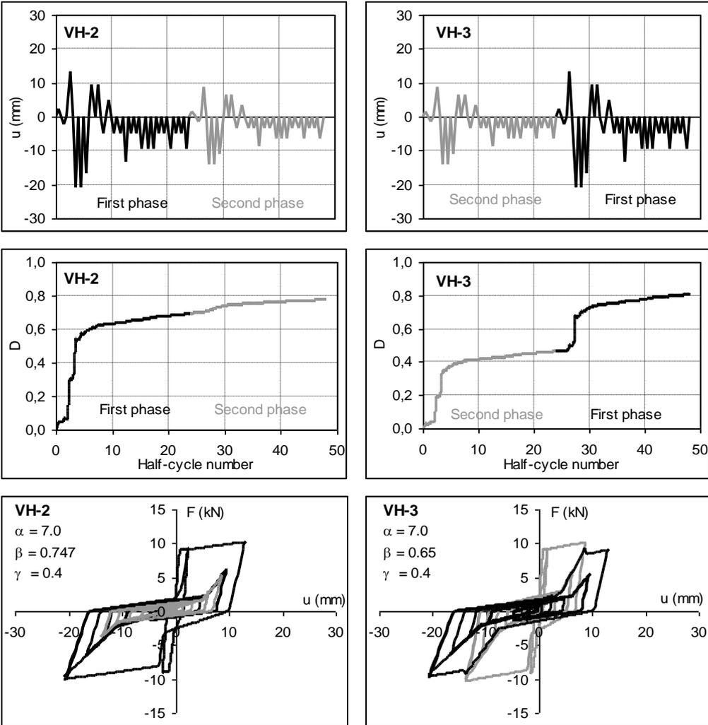
Figure 3.3. Loading histories, damage curves, force-displacement relationships of specimens VH-2 and VH-3
