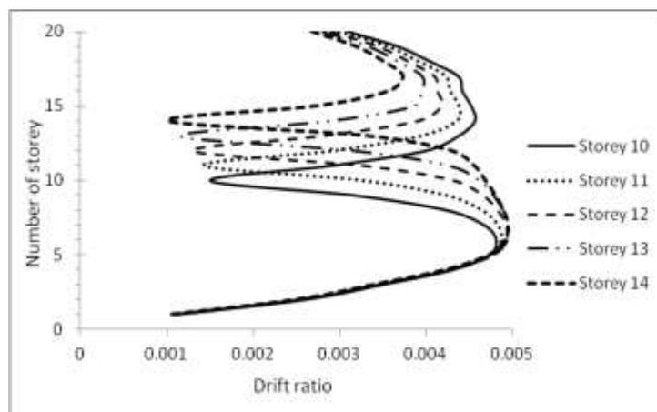
**Figure 6.** Drift ratios of 20 storey model obtained from RSA
