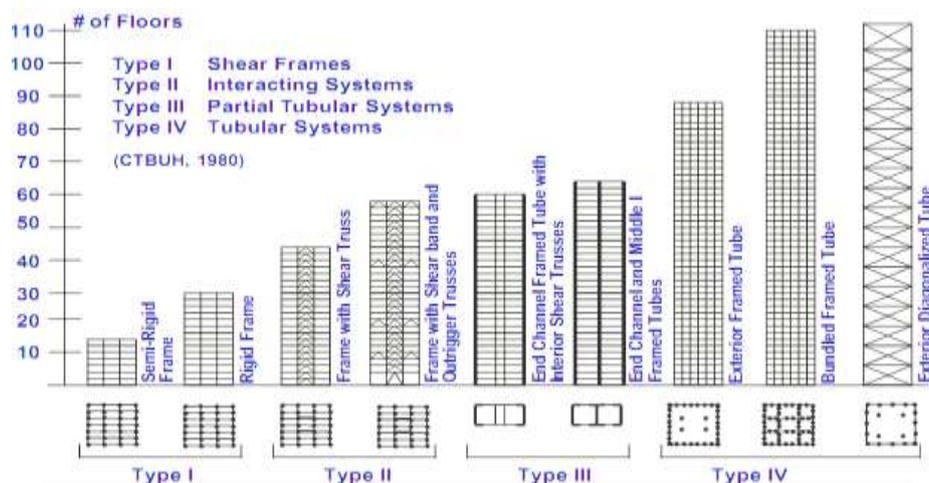
Figure 1. Evolution of structural systems
