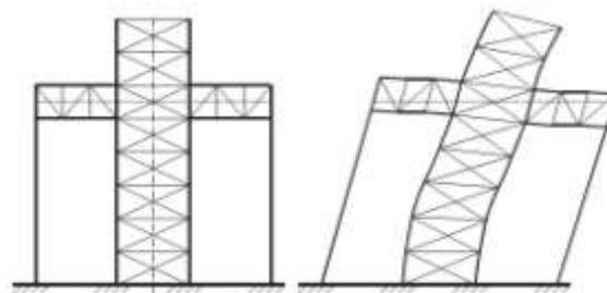
**Figure 3.** Performance of outrigger system against lateral load (Hoenderkamp, 2003)
