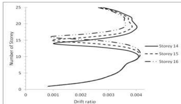
**Figure 8.** Drift ratios of 25 storey model obtained from RSA
