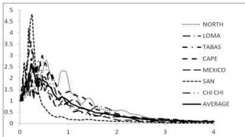
**Figure 5.** Spectra of utilized ground motions
