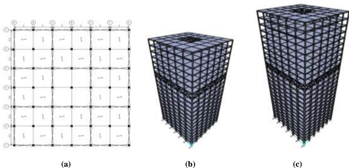
**Figure 4.** Geometric specifications: a) Floor plan (b) 20 storey model (c) 25 storey model
