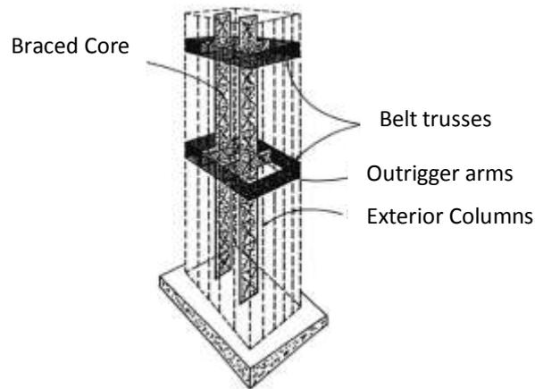
**Figure 2.** Structural schematic of tall building with outrigger and belt truss (Taranath, 1988)
